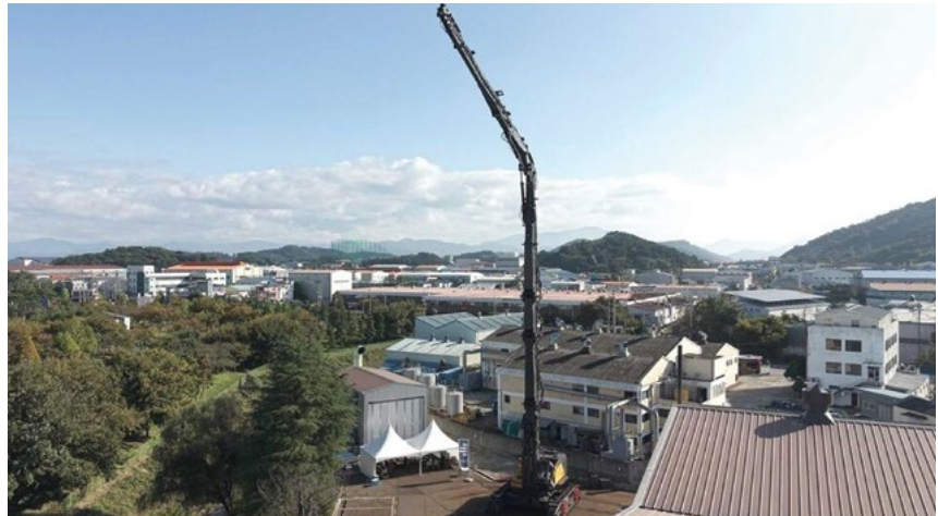
The EC950 High Reach is the largest high-reach excavator from Volvo Construction Equipment.
