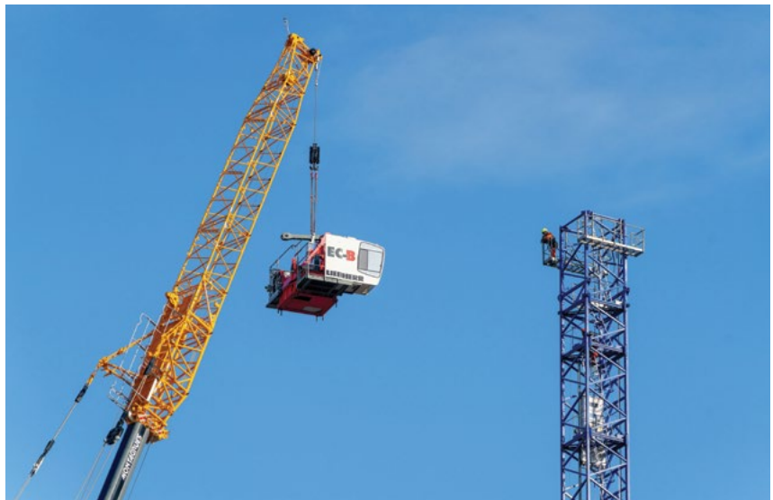
The slewing ring and cab hang on the hook of the LTM 1400-6.1. The fixed lattice jib of the new 400 t crane can be set up to a length of 45.5 m. The longest luffing jib measures an impressive 80.5 m. This enables the mobile crane to reach lifting heights of up to 120 m.
