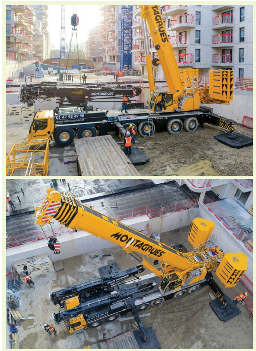
With a single lift, the LTM 1400-6.1 places the Y-guying system on its undercarriage and can then attach it fully automatically to the telescopic boom by luffing it down, using the Solidlink quick coupling.
