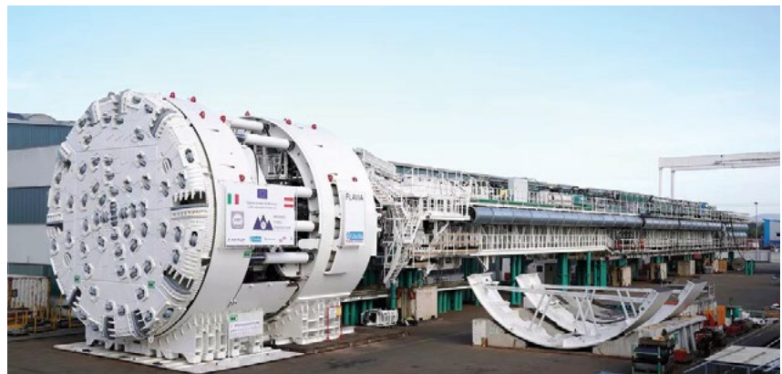
One of the Double Shield TBMs from Herrenknecht, used for excavation of the western tube of the Brenner Base Tunnel on the Italian side.
