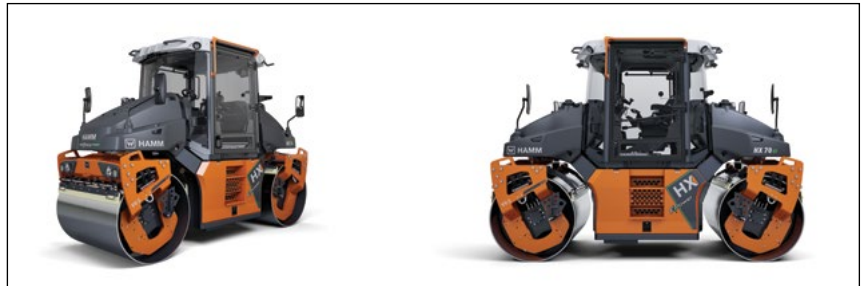
The HX 70e pivot-steered tandem rollers deliver the same compaction power as the diesel-powered models of the HX series.
