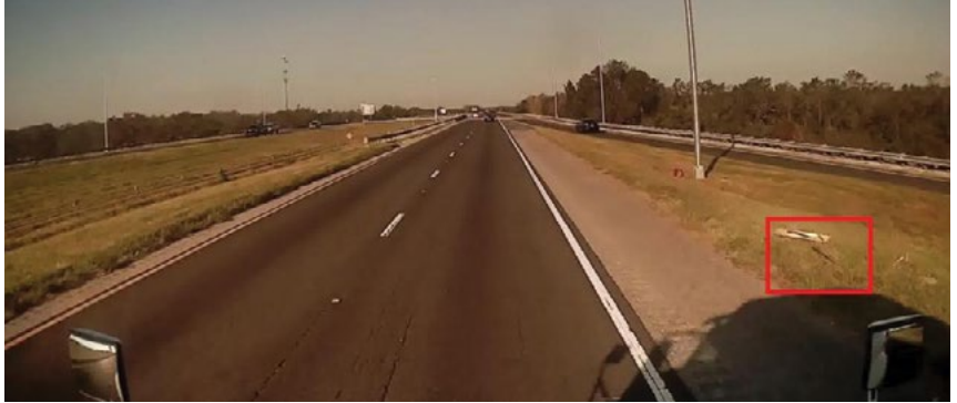
Bentley's Blynscsy AI technology detects a broken highway sign after Hurricane Helene in Florida. Image: Bentley Systems.
