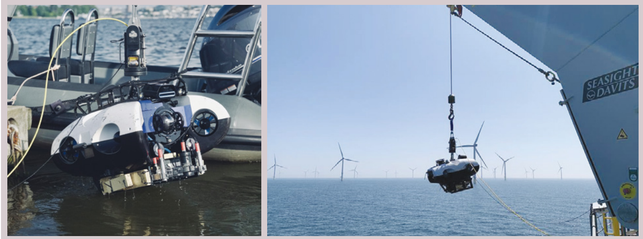
BeeX's flagship Hovering Autonomous Underwater Vehicle (HAUV), A.IKANBILIS, used for underwater inspections Images: BeeX.
