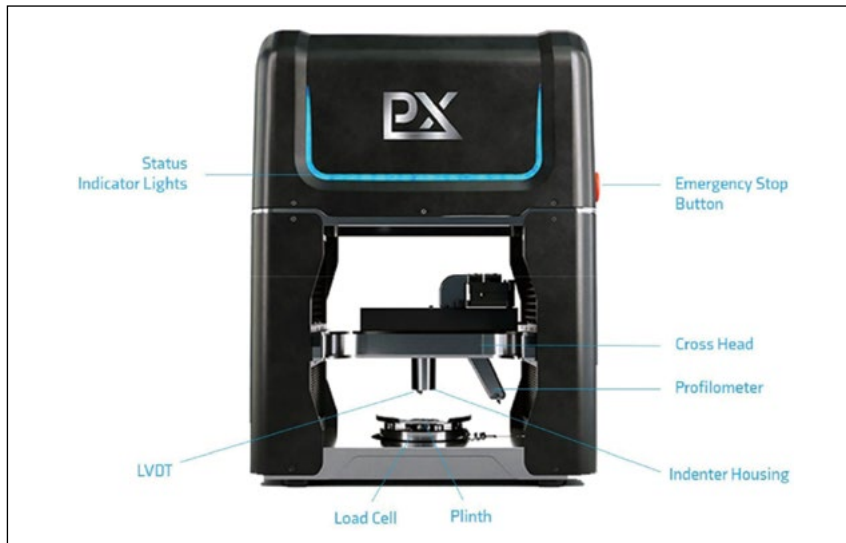
The benchtop plastometer from Plastometrex. Image: Plastometrex.
