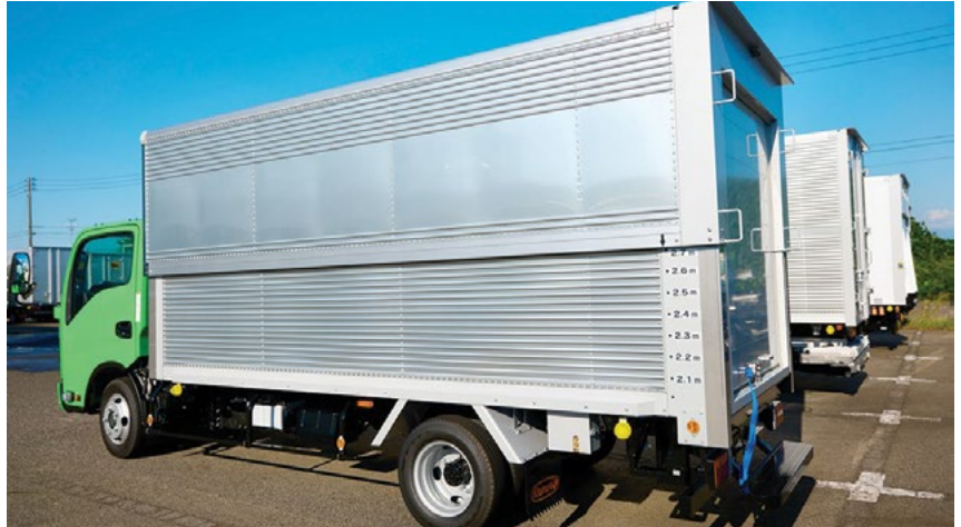
The 'Limbo Van' is one of Kitamura Manufacturing's iconic products, used by large delivery companies. The height of the loading platform can be adjusted depending on the weight of cargo or the height of the loading bay.
