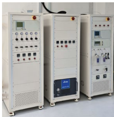
Figure 6: Fourier Transform Infrared Spectroscopy (FTIR) test equipment at A*STAR's Battery Centre.
