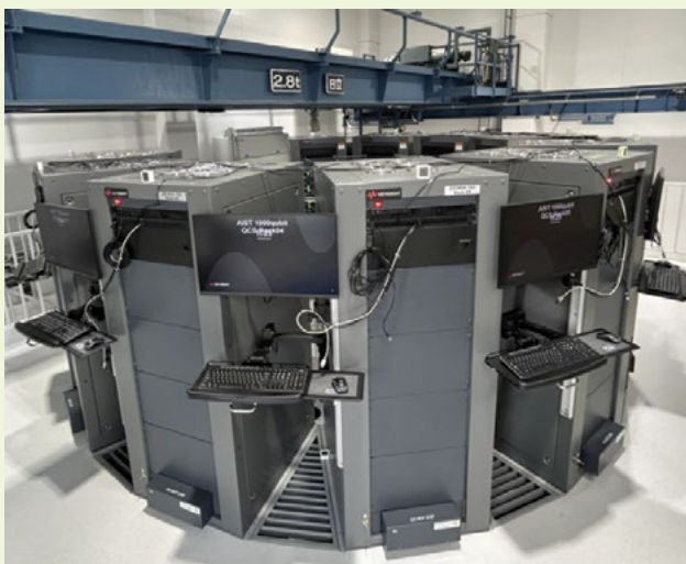
Keysight's 1,000-qubit quantum control system solution installed at the National Institute of Advanced Industrial Science and Technology (AIST) in Tsukuba, Japan.
