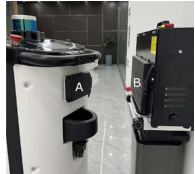
The Phoenix wireless charger mounted on a cleaning robot. The receiver is labelled 'A' while the transmitter is labelled 'B'.
