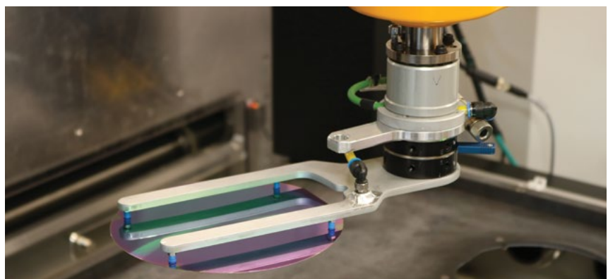
The flat vacuum gripping system, which can be quickly exchanged for the different sized wafers, maintains the specified positioning accuracy of \pm 0.1 mm when loading the workpiece carriers.
