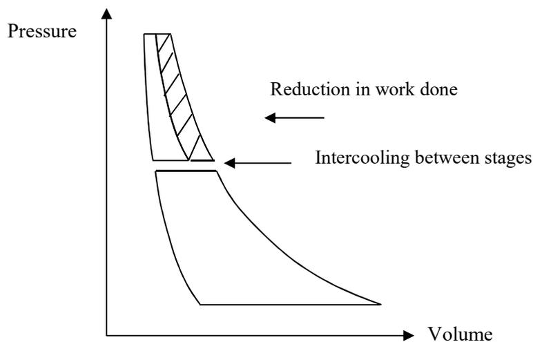
Figure 10.2 P-V diagram for two stage compression
