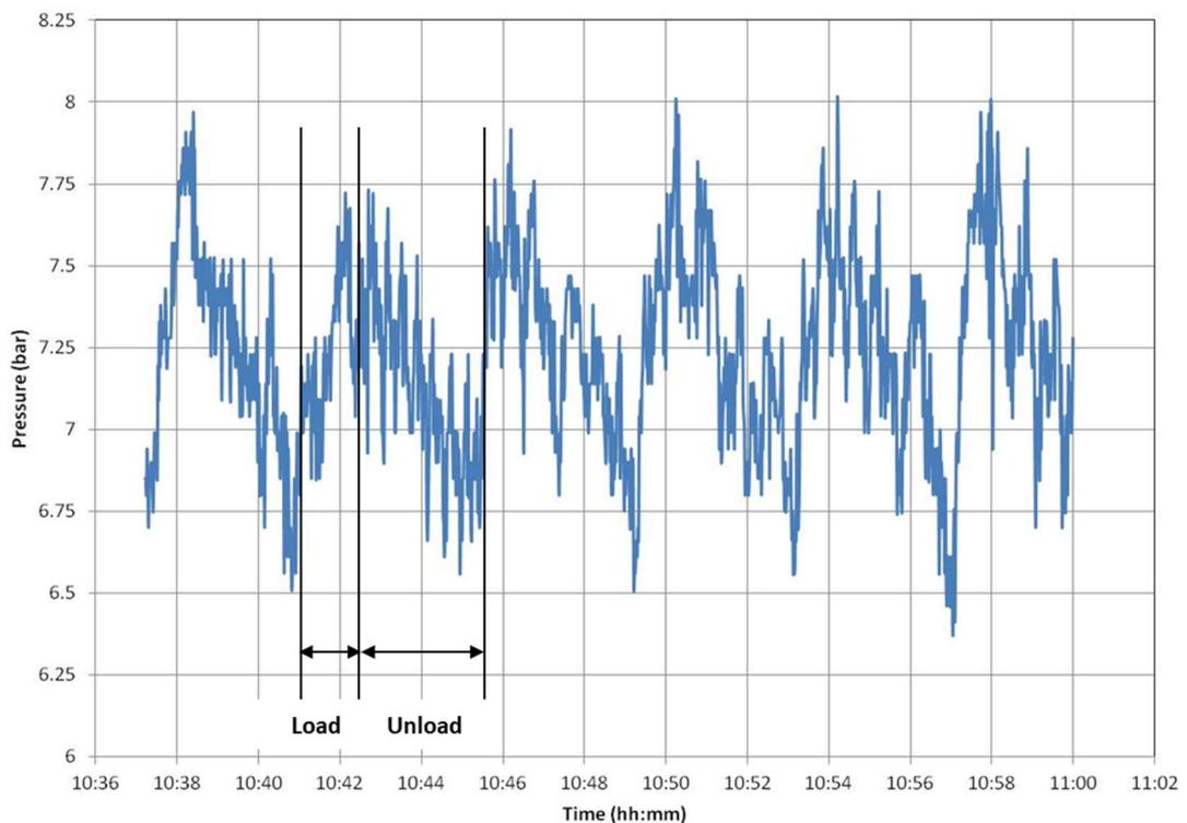
Figure 11.5 Plot showing compressor loading and unloading time
