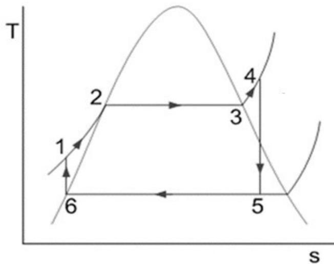
Figure 3.13 T-S diagram for steam turbine
