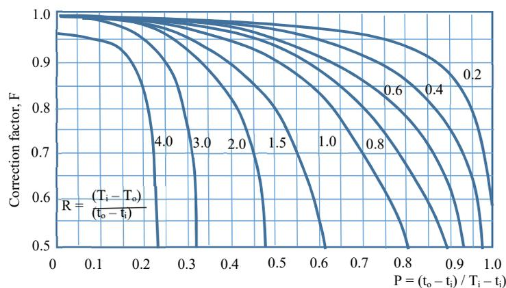
Figure 13.6 Correction factor F when both fluids are unmixed
