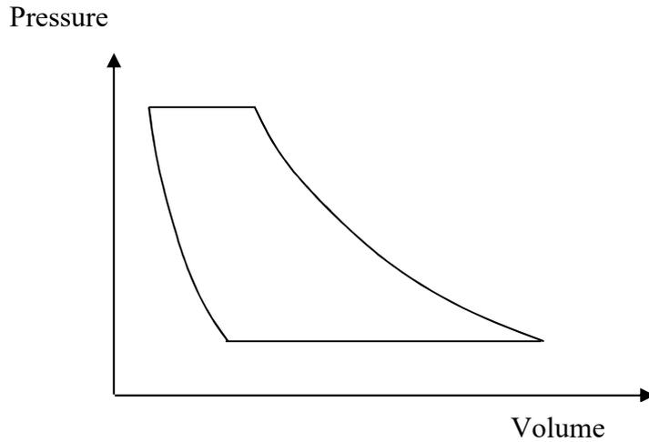
Figure 10.1 P-V diagram for single stage compression
