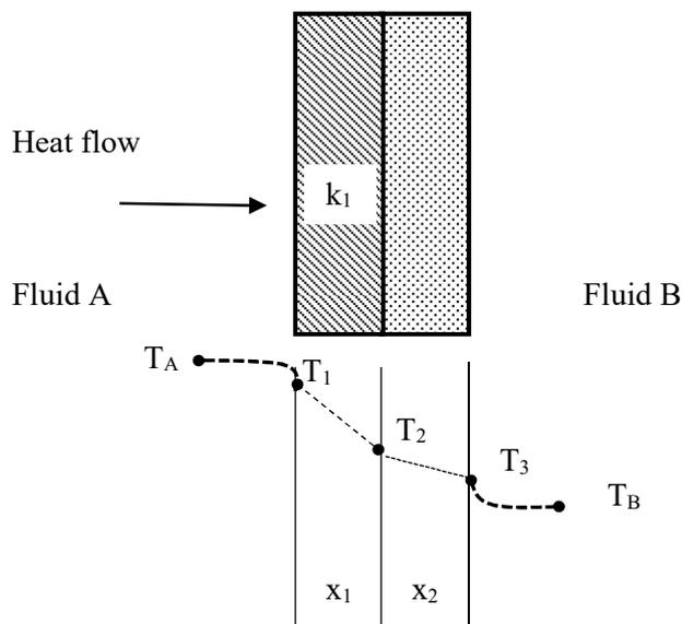
Figure 12.7 Heat transfer across a composite material
