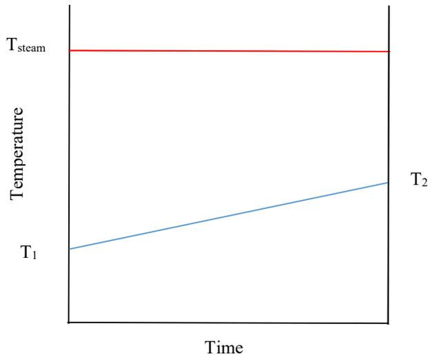
Figure 3.9 Temperature profile for flow-type heating
