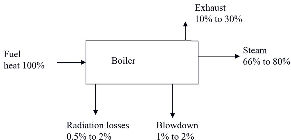
Figure 2.9 Typical heat balance for a boiler
