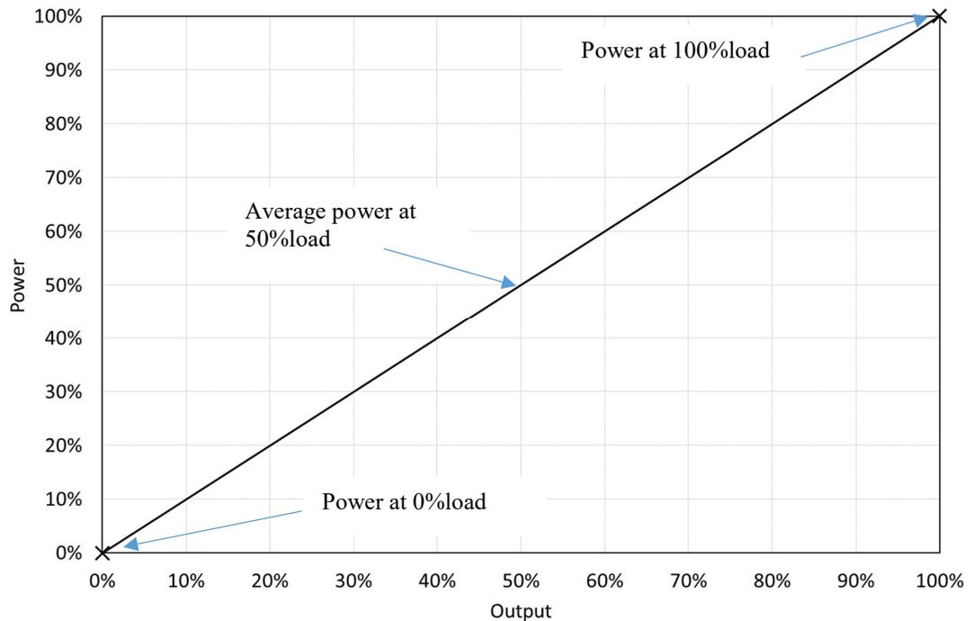
Figure 9.2 Output vs power for on / off control
