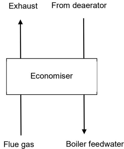
Figure 12.2 Typical heat recovery system for boiler exhaust
