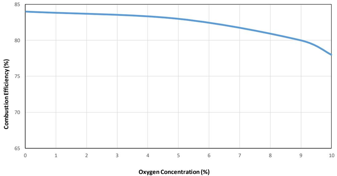
Figure 4.1 Combustion efficiency versus O<sub>2</sub> concentration (courtesy of Cleaver-Brooks)
