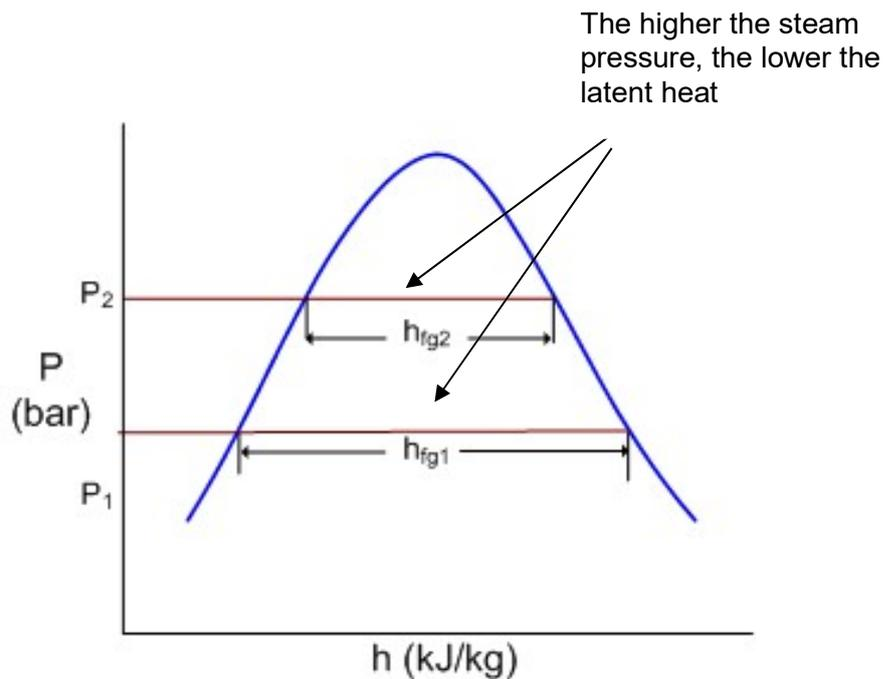
Figure 4.3 Change in latent heat with change in steam pressure
