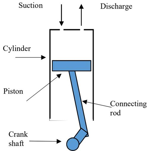
Figure 6.7 Image of a single-stage reciprocating compressor.
