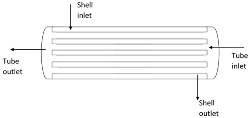
Figure 14.1 One shell pass and one tube pass
