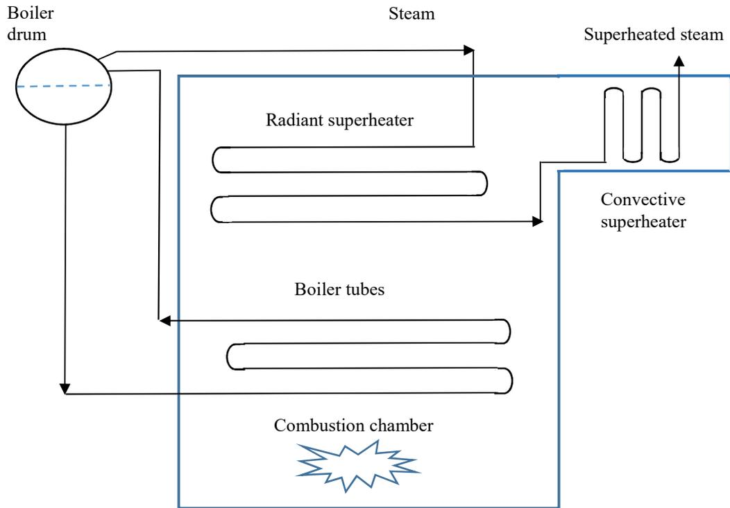
Figure 2.6 Arrangement of radiant and convective superheaters
