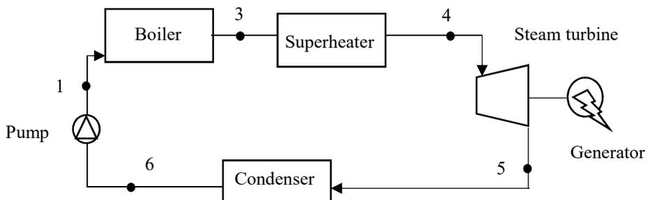
Figure 3.12 Arrangement of a steam turbine power generation plant
