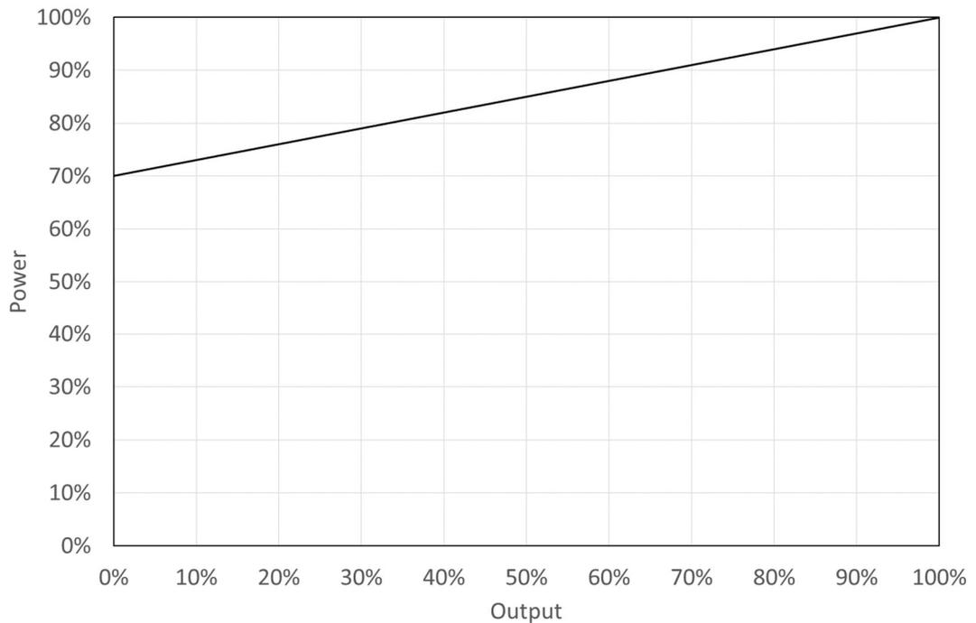
Figure 9.6 Output vs power for inlet modulation control
