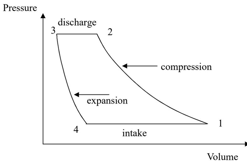
Figure 8.2 Typical Compression process
