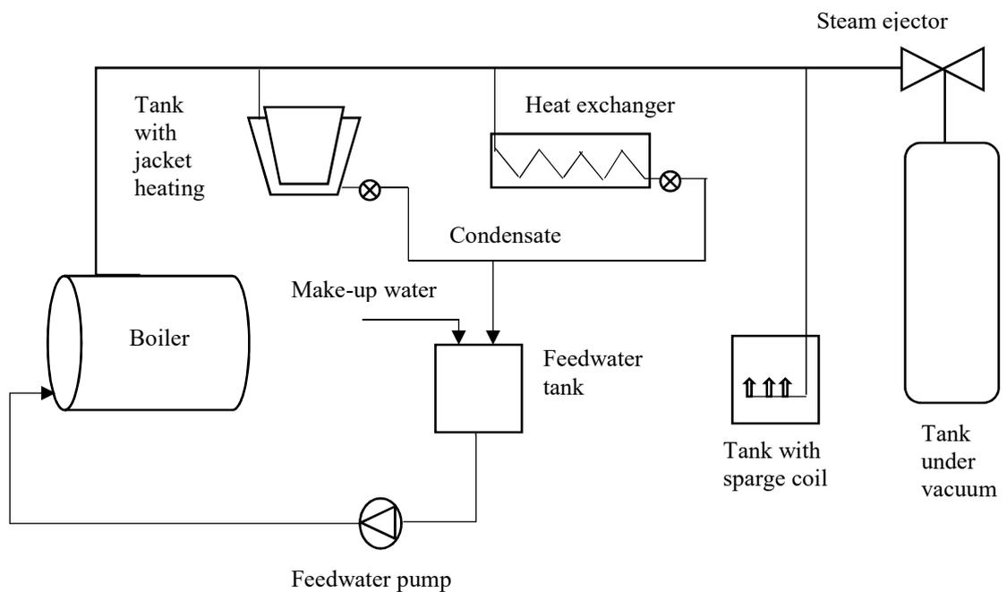
Figure 3.1 A typical steam distribution system
