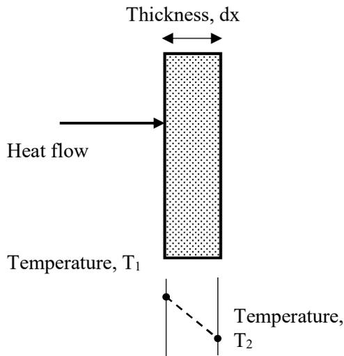
Figure 12.3 Heat transfer by conduction
