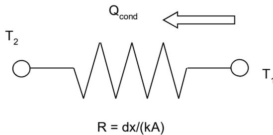
Figure 12.4 Thermal analogy of Ohm's law
