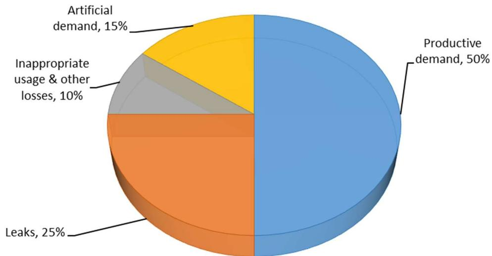
Figure 6.2 Typical breakdown of compressed air usage (Ref. 4)
