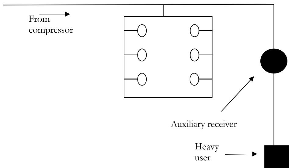
Figure 7.10 Arrangement of an auxiliary receiver to reduce pipe velocity
