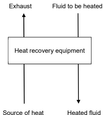
Figure 12.1 Arrangement of a heat recovery system
