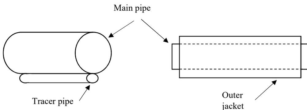
Figure 3.10 Arrangement of steam tracing
