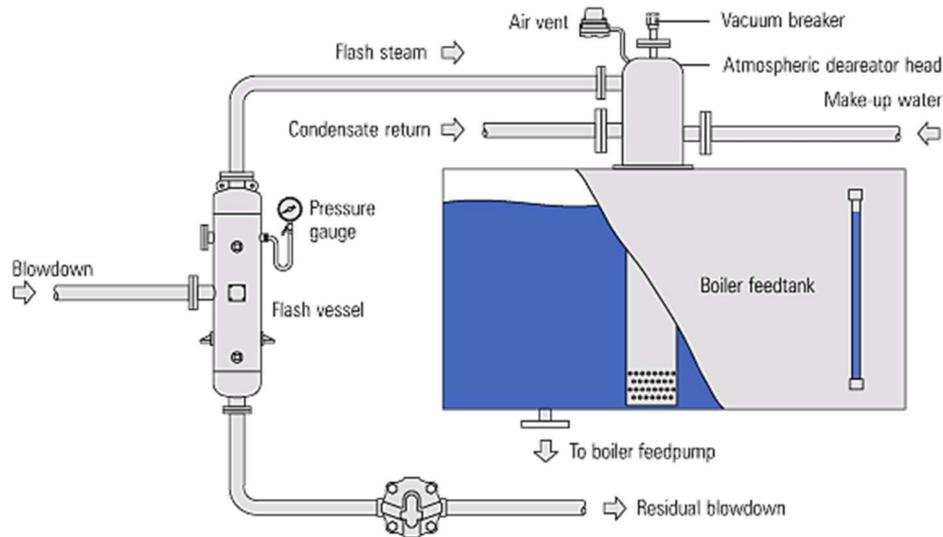
Figure 4.10 Typical blowdown flash steam recovery system (illustration taken from the Spirax Sarco website 'Steam Engineering Tutorials' at <http://www.spiraxsarco.com>)
