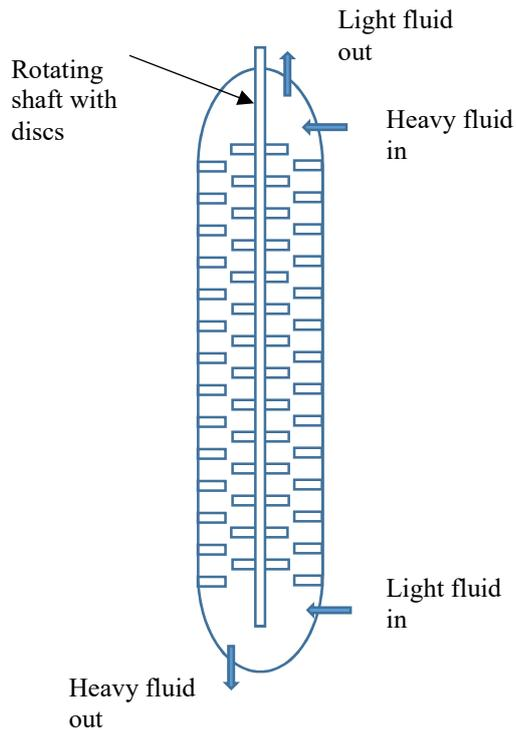
Figure 14.14 Arrangement of a mechanically agitated tower
