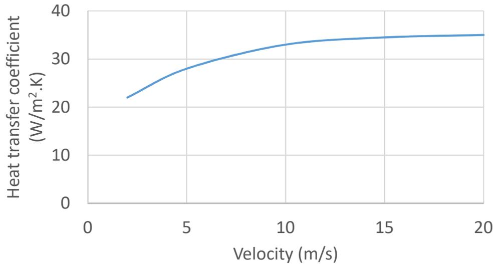
Figure 12.8 Convective heat transfer coefficient values at different air velocities
