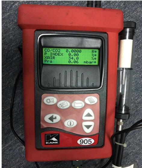
Figure 2.11 A combustion analyser
