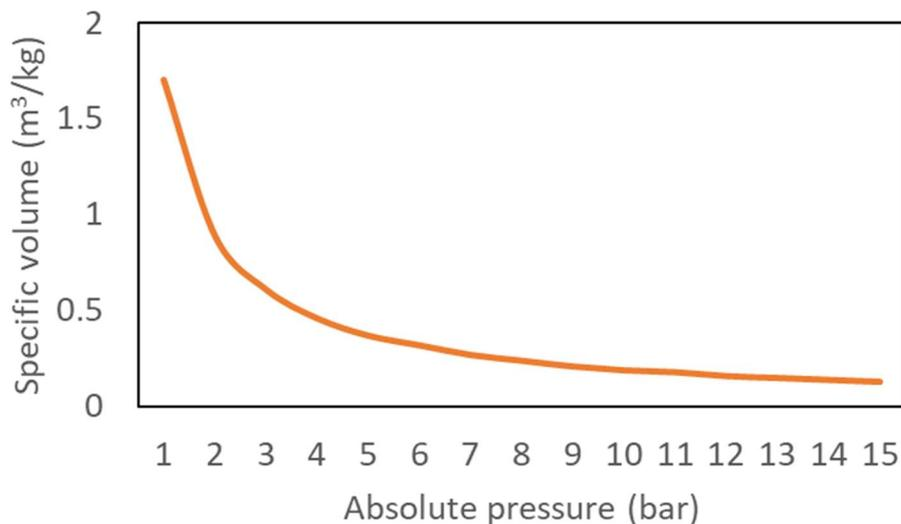
Figure 1.4 Steam pressure vs specific volume
