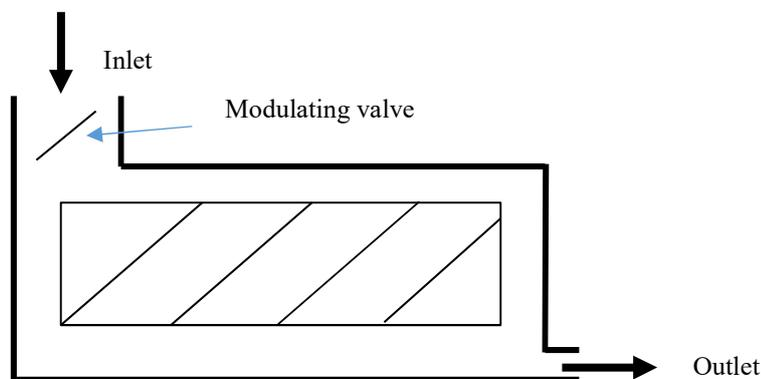
Figure 9.5 Inlet modulation of a screw compressor
