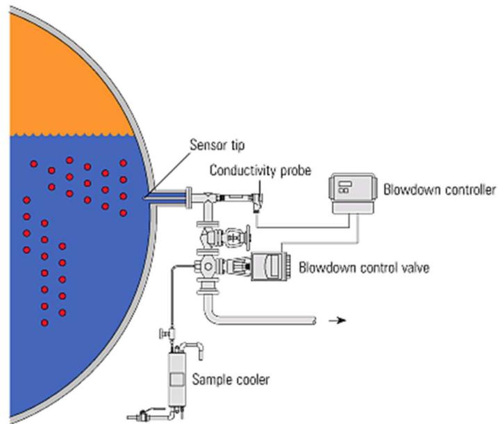
Figure 4.8 Typical arrangement of automatic blowdown control (illustration taken from the Spirax Sarco website 'Steam Engineering Tutorials' at <http://www.spiraxsarco.com>)
