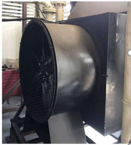
Figure 7.8 Image of an air-cooled intercooler
