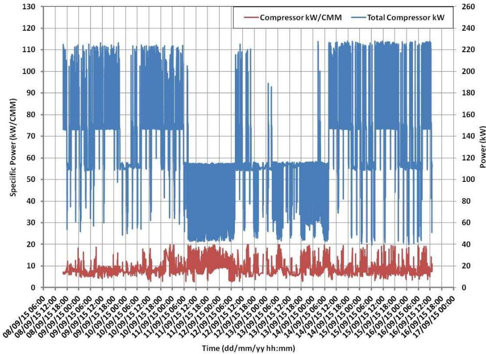
Figure 11.4 Typical plot of compressor power and specific power
