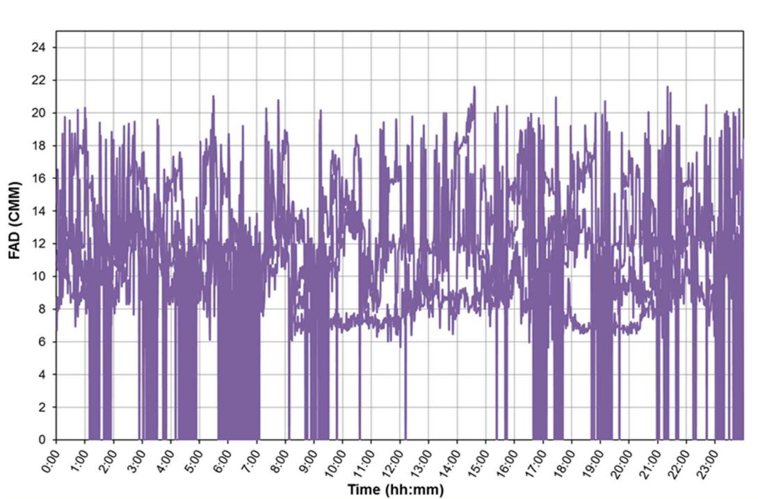
Figure 11.6 Compressed air FAD profile
