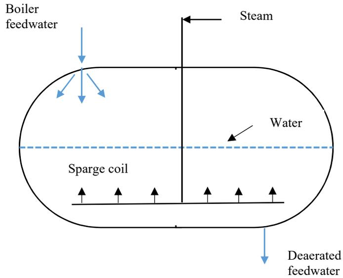
Figure 2.7 Arrangement of a spray type deaerator
