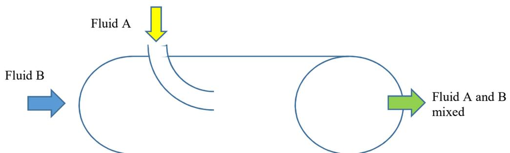
Figure 14.13 Arrangement of a turbulent pipe contactor
