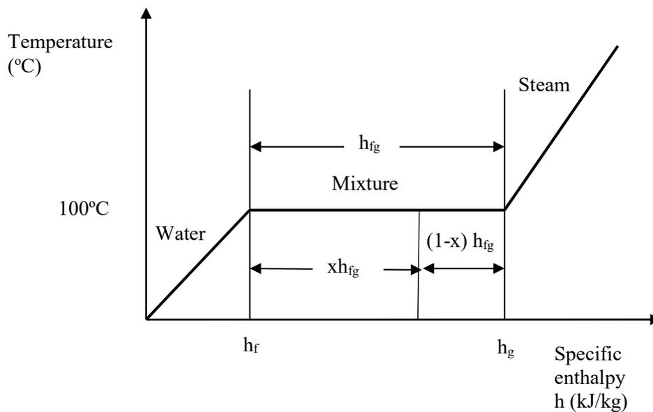
Figure 1.5 Relationship between temperature and enthalpy
