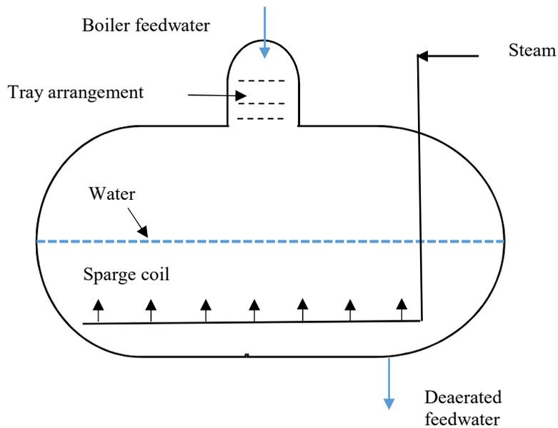
Figure 2.8 Arrangement of a tray type deaerator
