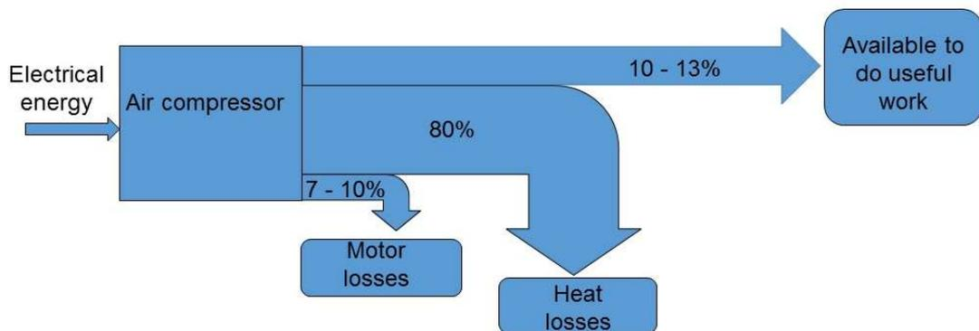
Figure 6.1 Energy flow for a compressed air system
