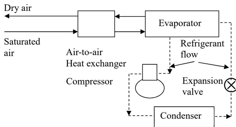
Figure 7.1 Arrangement of a refrigerant dryer
