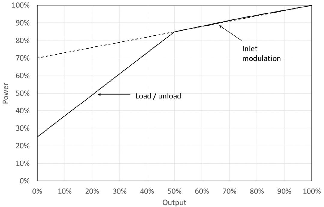
Figure 9.7 Output vs power for inlet modulation followed by load / unload
