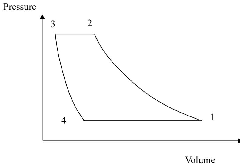
Figure 6.9 Compression process on a PV diagram
