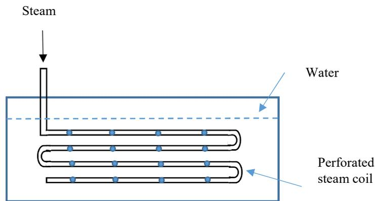
Figure 14.12 Direct contact type heat exchanger used for heating water
