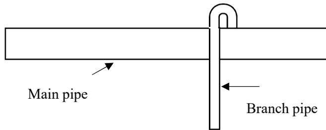
Figure 3.6 Recommended arrangement of a branch connection
