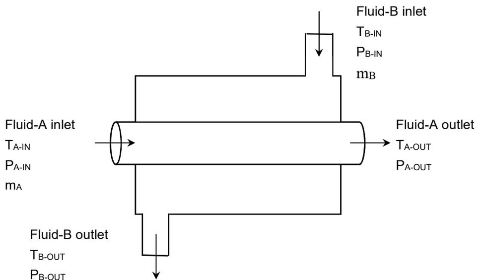
Figure 15.1 Measurement locations for a heat recovery system
