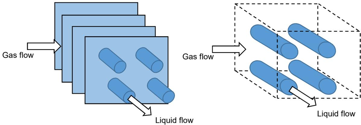
Figure 13.5 Arrangement of a cross-flow heat exchanger
