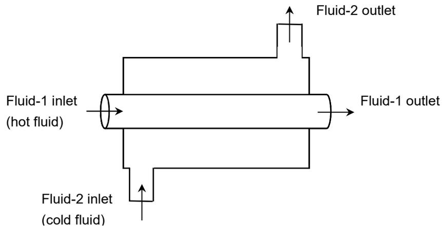
Figure 13.1 Arrangement of a parallel-flow heat exchanger
