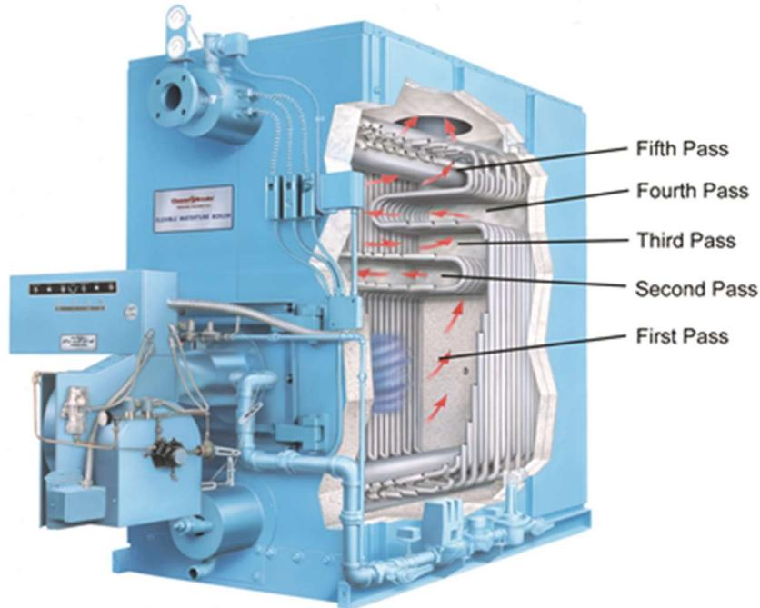
Figure 2.4 Cut-away of a commercial water tube boiler (courtesy of Cleaver-Brooks)
