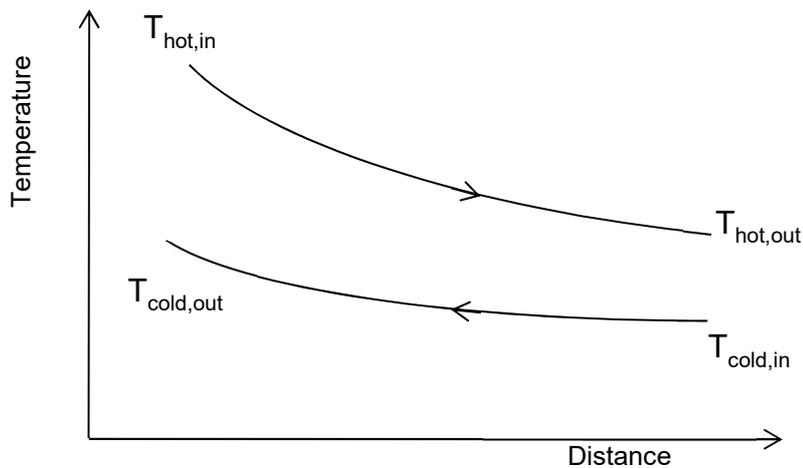
Figure 14.7 Heat exchanger fluid temperatures
