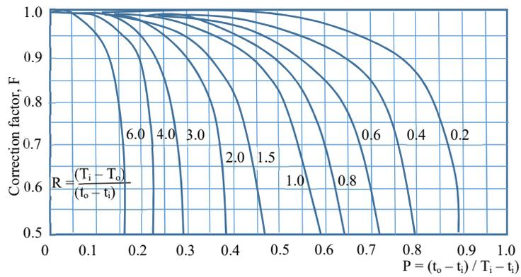
Figure 14.4 Correction factor F for one shell pass and multiple tube passes (multiples of 2)
