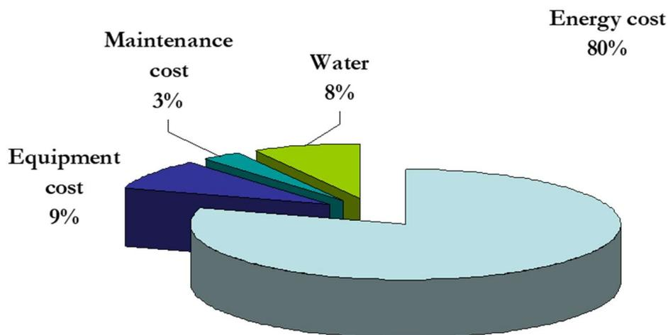
Figure 6.3 Typical lifecycle cost breakdown for an air compressor
