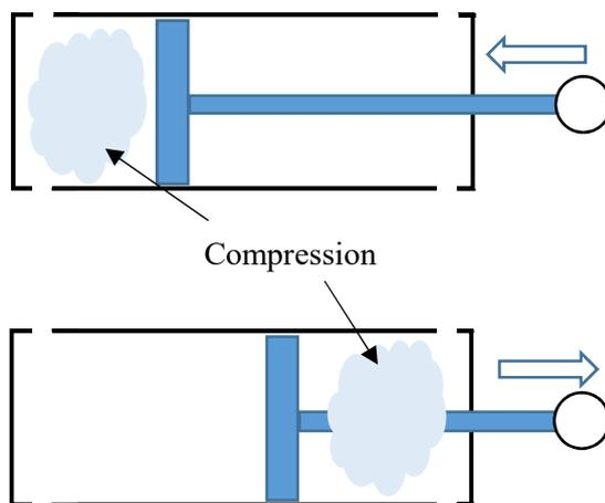
Figure 6.9 Arrangement of a double-acting reciprocating compressor
