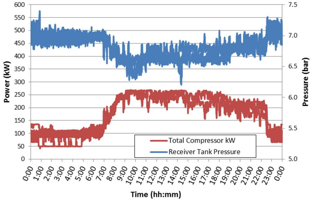
Figure 11.2 Pressure and compressor power profiles
