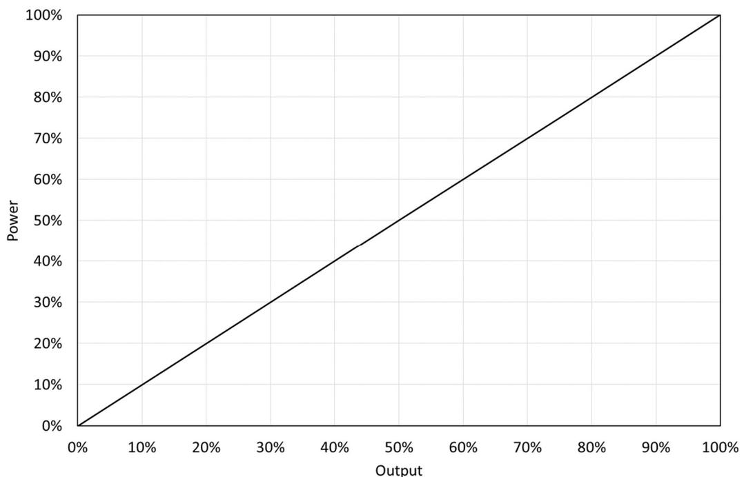
Figure 9.1 Ideal output vs power relationship for an air compressor
