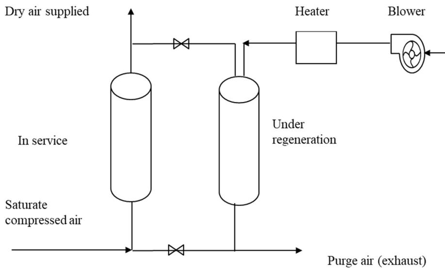
Figure 7.4 Arrangement of a desiccant dryer with external blower & heater
