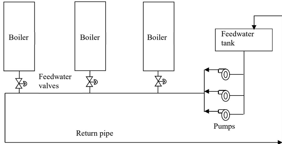
Figure 4.4 Feedwater pump arrangement for a multiple boiler operation
