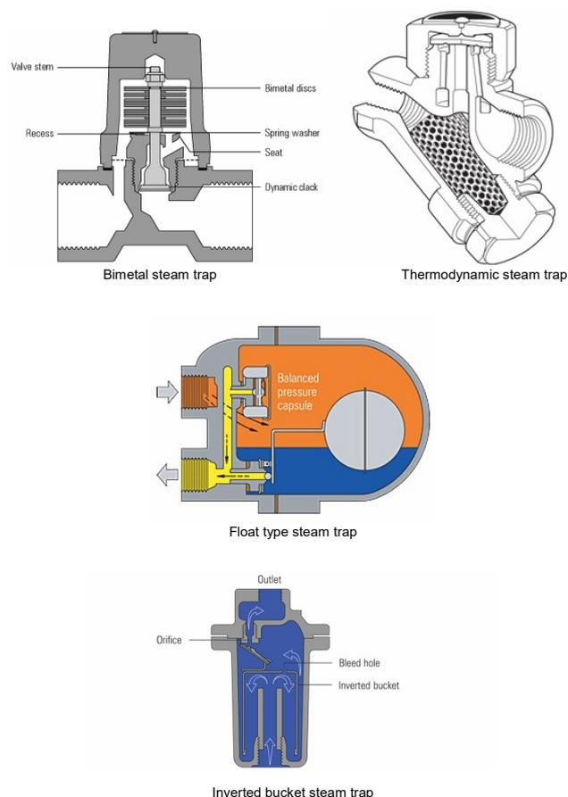
Figure 3.8 Common types of steam traps (images taken from the Spirax Sarco website 'Steam Engineering Tutorials' at <http://www.spiraxsarco.com>)
