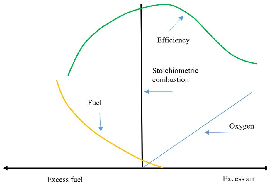
Figure 2.10 Excess air vs combustion efficiency
