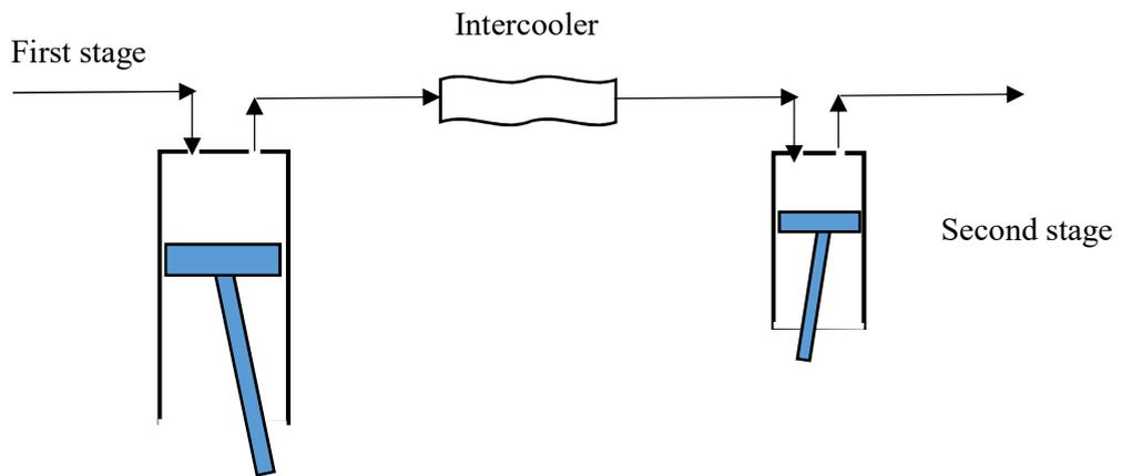
Figure 6.8 Arrangement of a two-stage reciprocating compressor.
