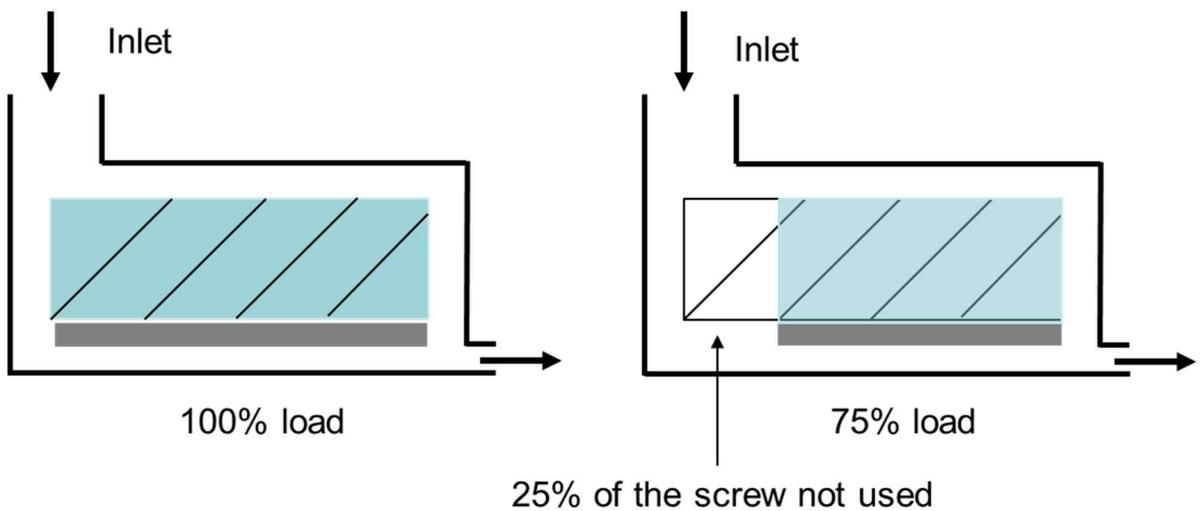
Figure 9.8 Variable displacement control at 100% and 75% loading
