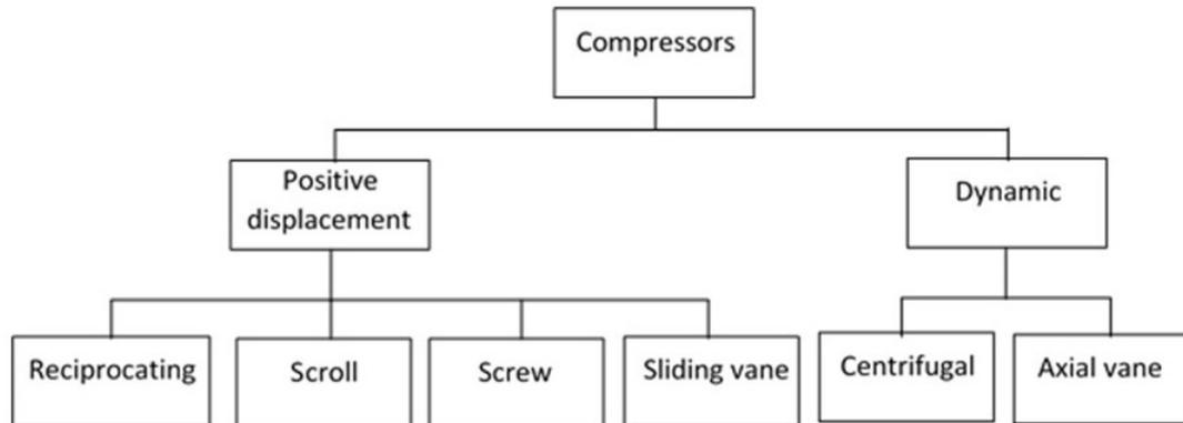
Figure 6.6 Different types of compressors
