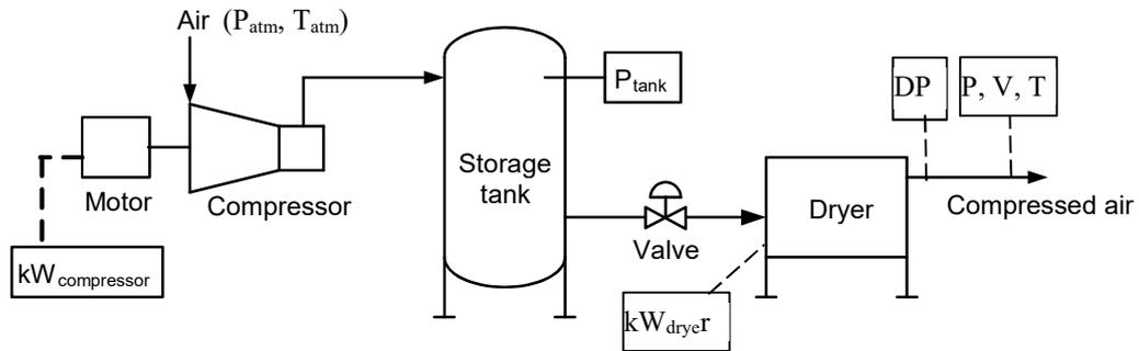
Figure 11.1 Measurement locations for a compressed air system
