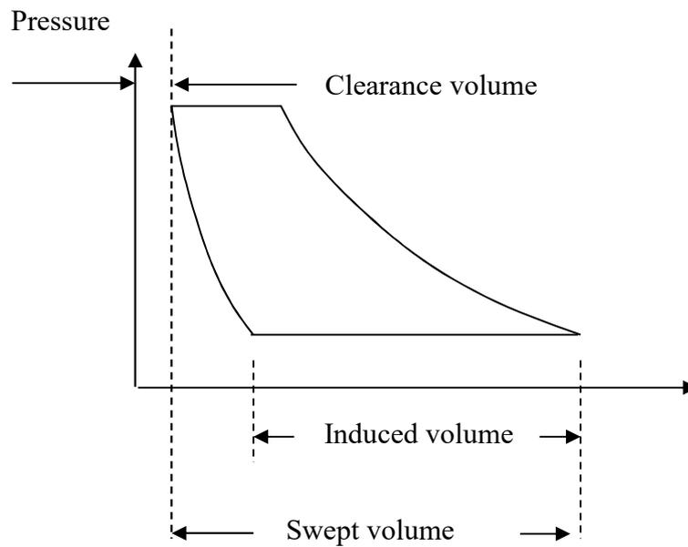
Figure 8.5 Illustration of volumetric efficiency
