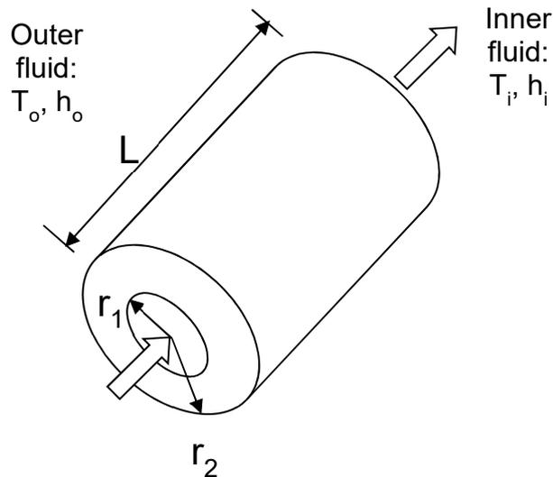
Figure 12.8 Heat transfer through an annular surface
