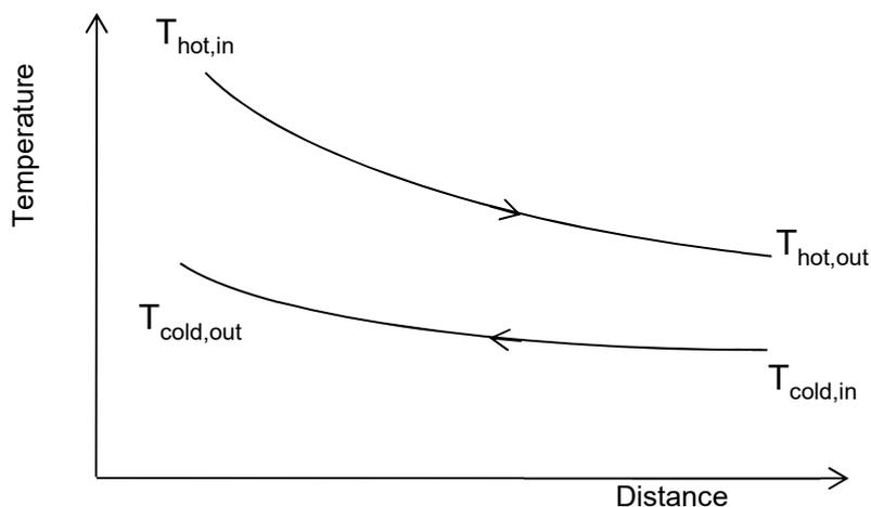
Figure 13.13 Typical fluid temperature profiles for a counterflow heat exchanger
