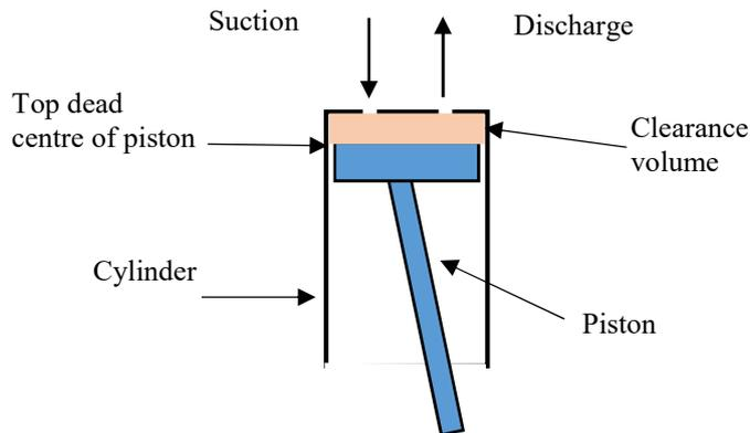
Figure 8.4 Illustration of clearance volume
