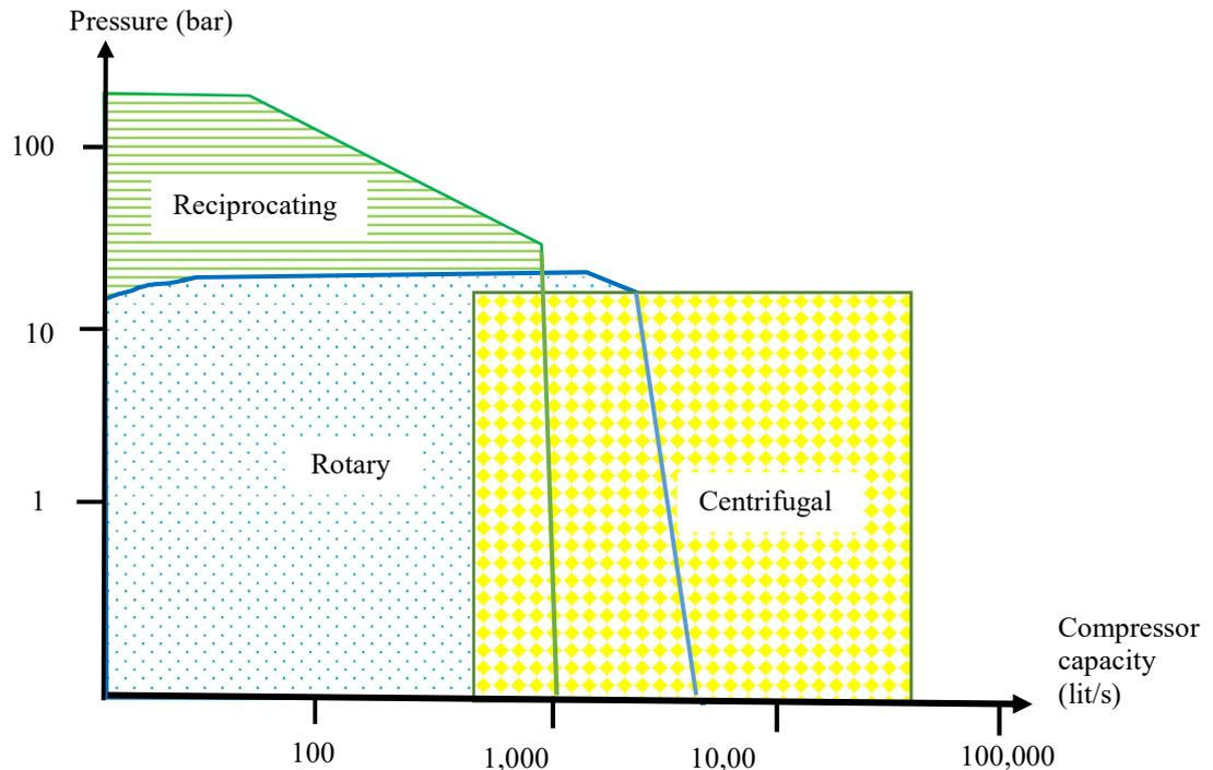
Figure 6.16 Operating range for common compressor types
