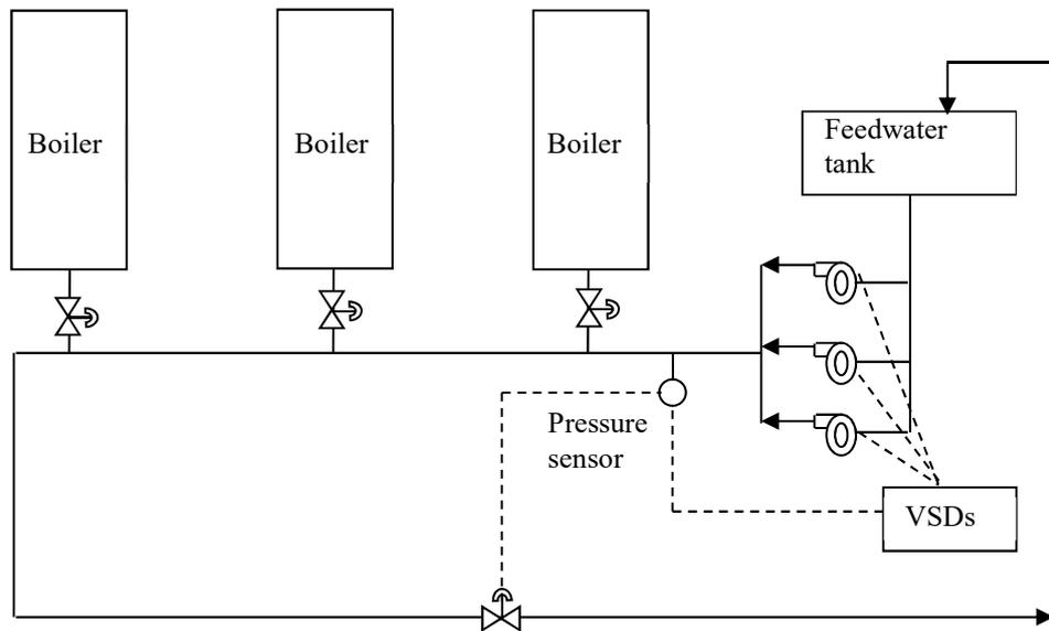
Figure 4.5 Suggested feedwater pump arrangement for a multiple boiler operation
