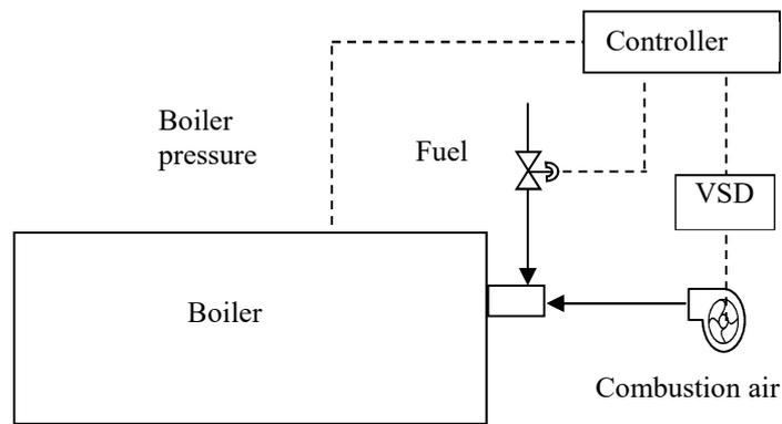
Figure 4.6 Application of VSD for boiler fan
