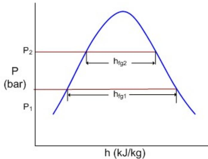
Figure 1.6 Enthalpy of evaporation at different pressures
