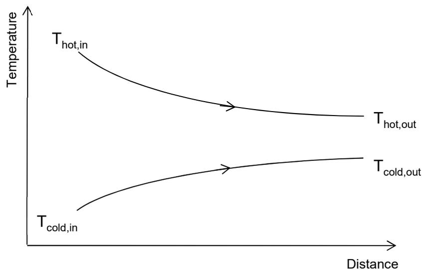
Figure 13.2 Temperature profile for a parallel-flow heat exchanger
