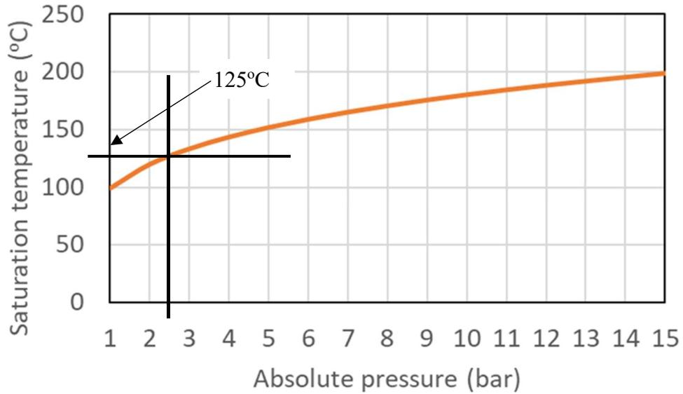
Figure 1.2 Steam temperature for Example 1.1
