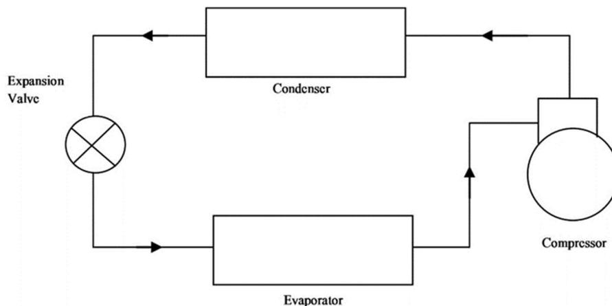
Figure 4.12 Vapour compression cycle used in hot water heat pumps
