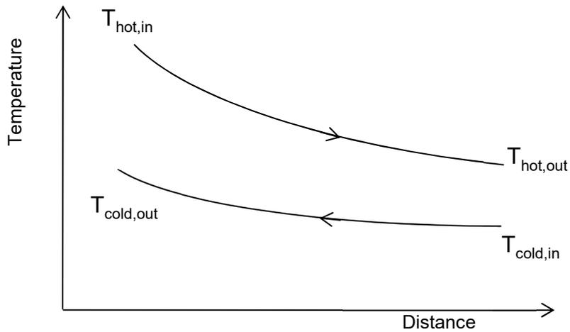
Figure 13.4 Temperature profile for a counter flow heat exchanger
