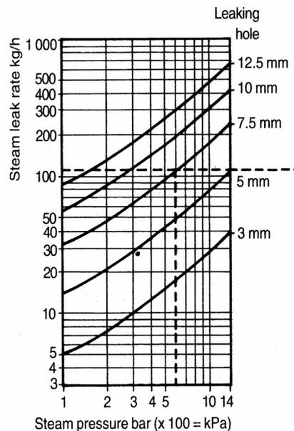
Figure 4.11 Steam losses through leaks (illustration taken from the Spirax Sarco website 'Steam Engineering Tutorials' at <http://www.spiraxsarco.com>)
