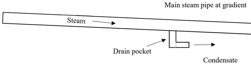
Figure 3.4 Recommended arrangement for steam mains
