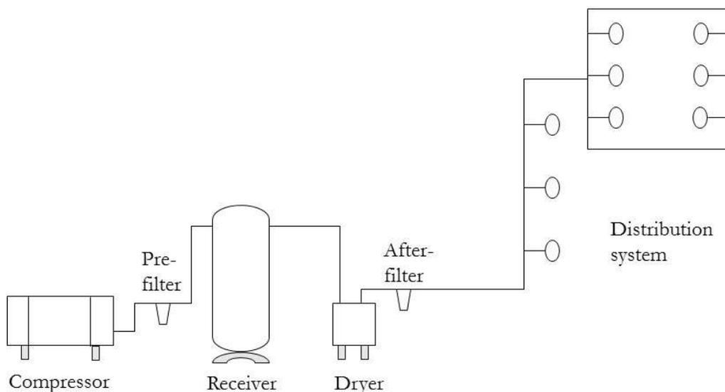
Figure 6.4 Arrangement of a typical compressed air system
