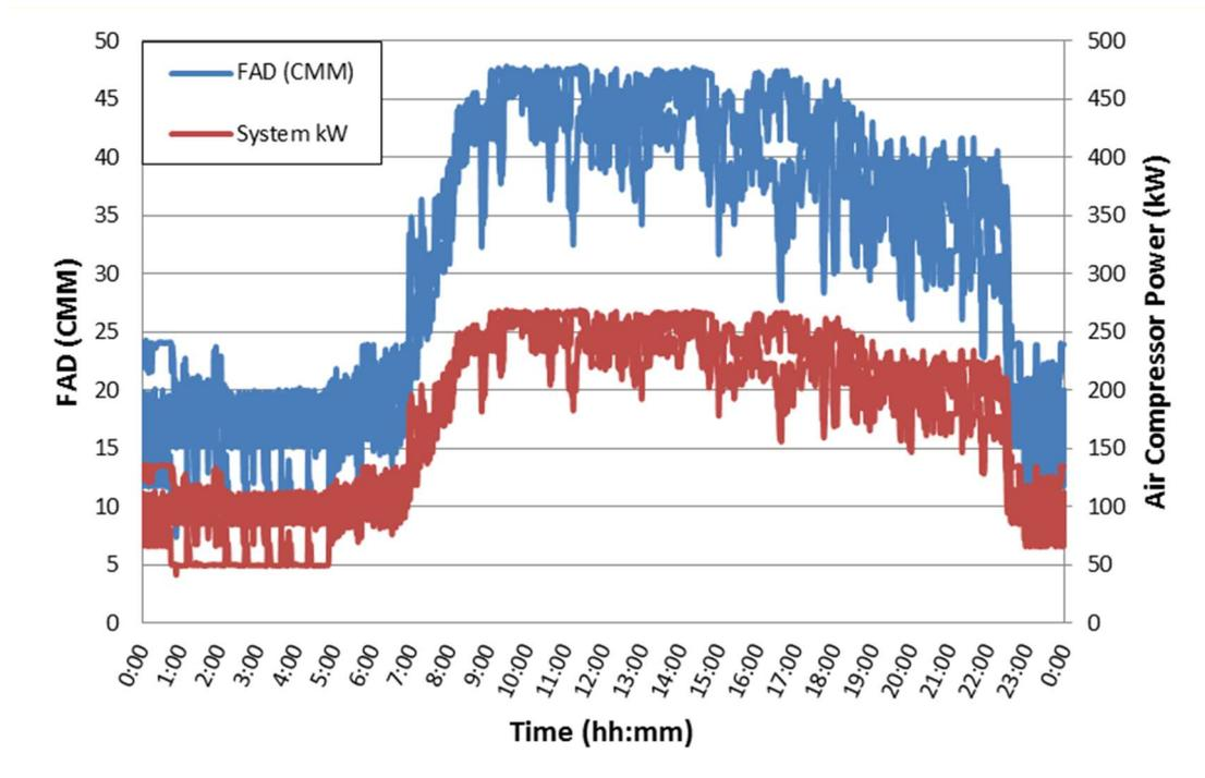
Figure 11.3 Typical FAD and compressor power profiles
