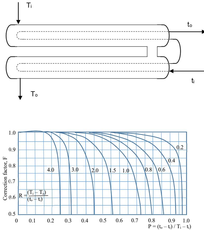
Figure 14.5 Correction factor F for two-shell pass and multiple tube passes (multiples of 4)
