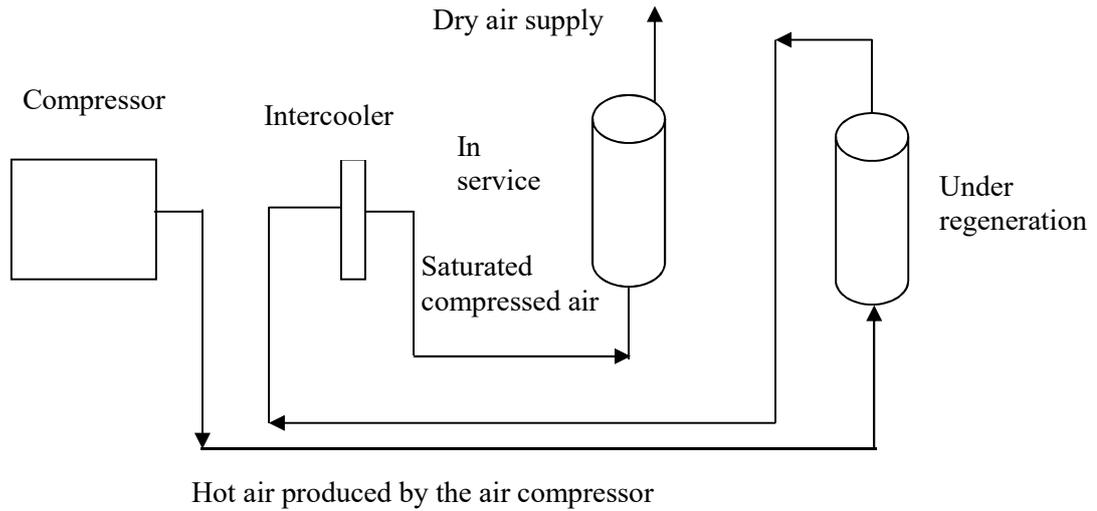
Figure 7.5 Arrangement of a heat of compression desiccant dryer
