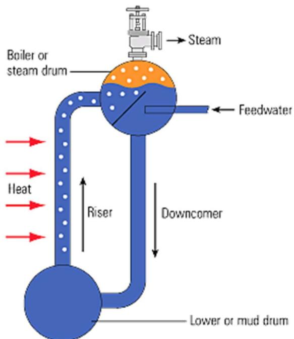
Figure 2.5 Water circulation in a water tube boiler (illustration taken from the Spirax Sarco website 'Steam Engineering Tutorials' at <http://www.spiraxsarco.com>)
