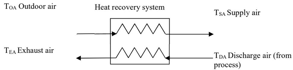
Figure 14.10 Heat exchange in a rotary heat exchanger
