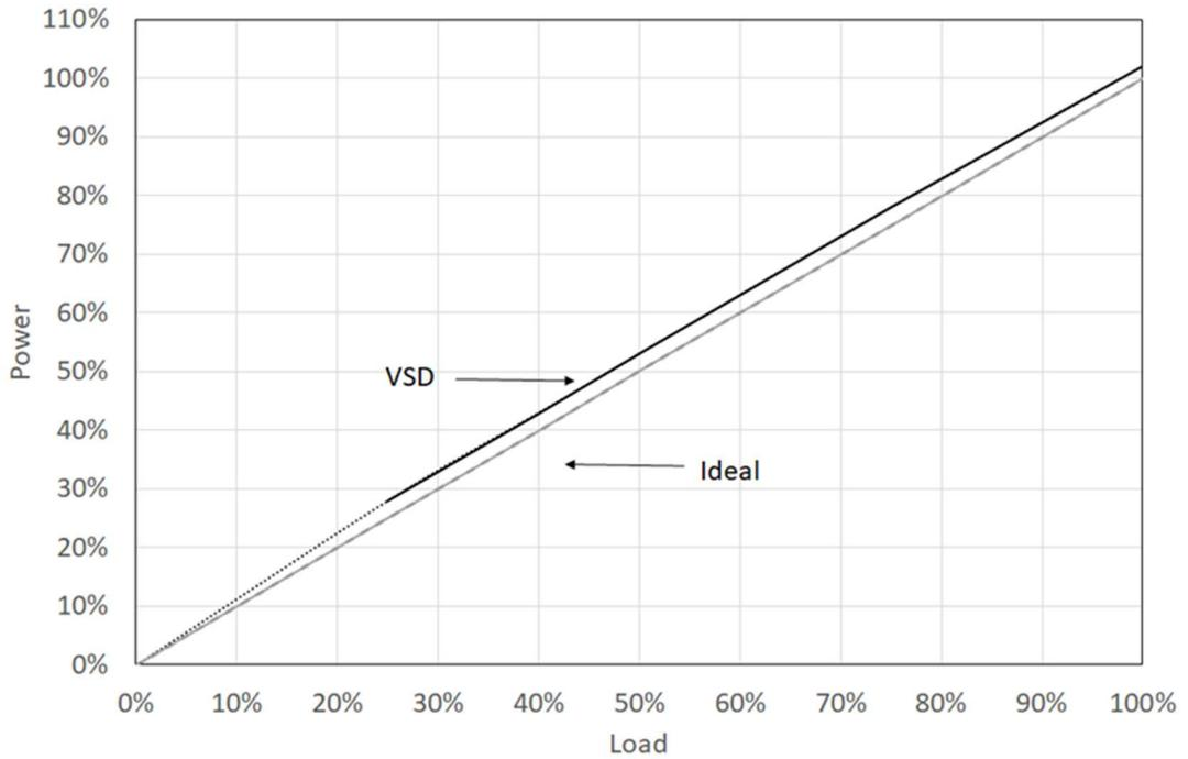
Figure 9.10 Output vs power for VSD compressor
