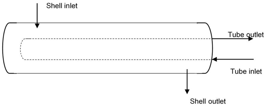
Figure 14.2 One shell pass and two tube passes
