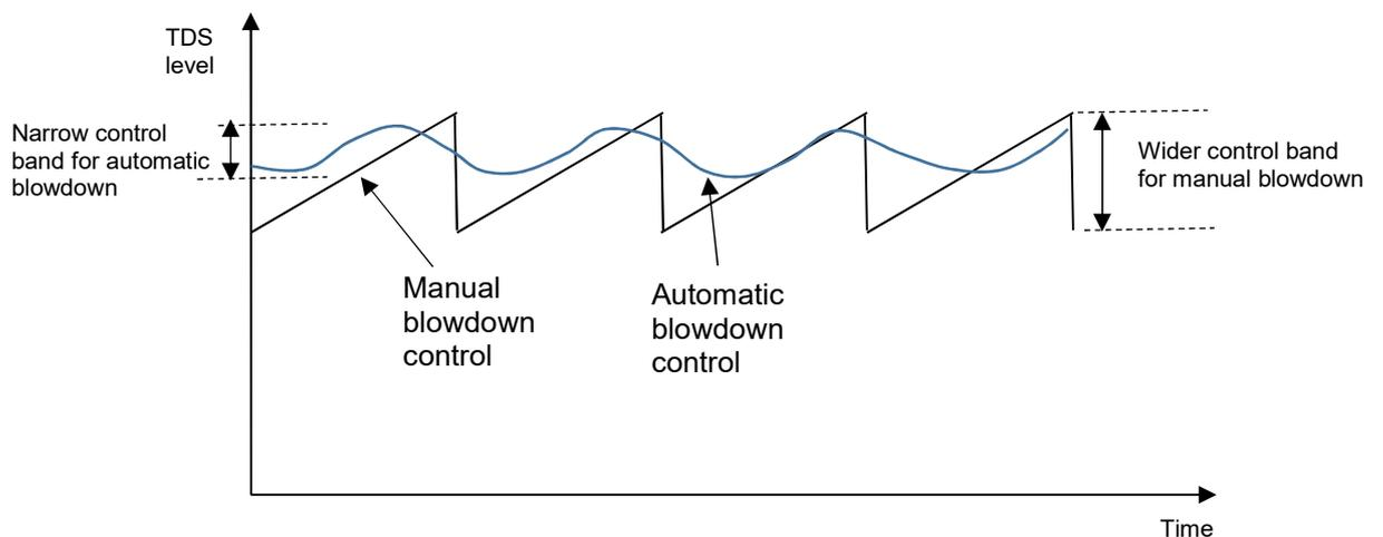
Figure 4.9 Comparison of TDS level for automatic and manual blowdown
