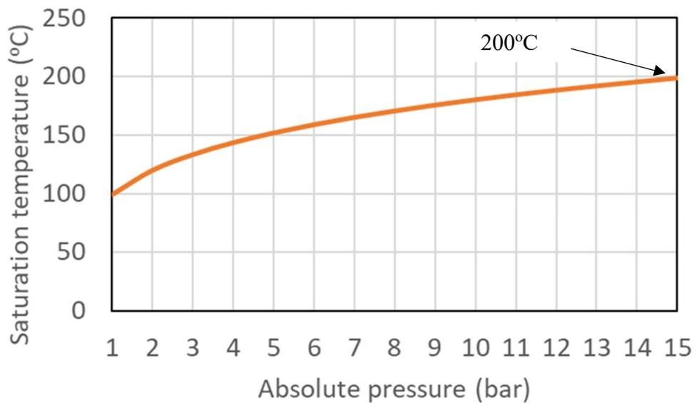
Figure 1.3 Steam temperature for Example 1.2
