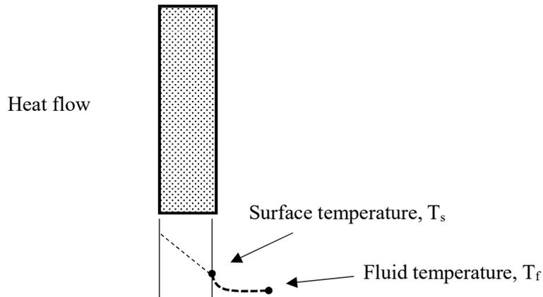
Figure 12.5 Convective heat transfer at the inner surface
