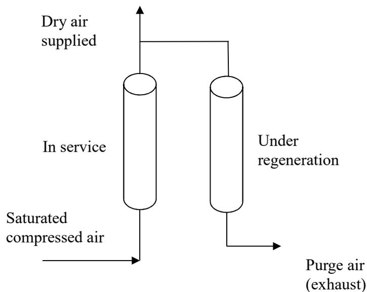
Figure 7.3 Arrangement of a heatless desiccant dryer
