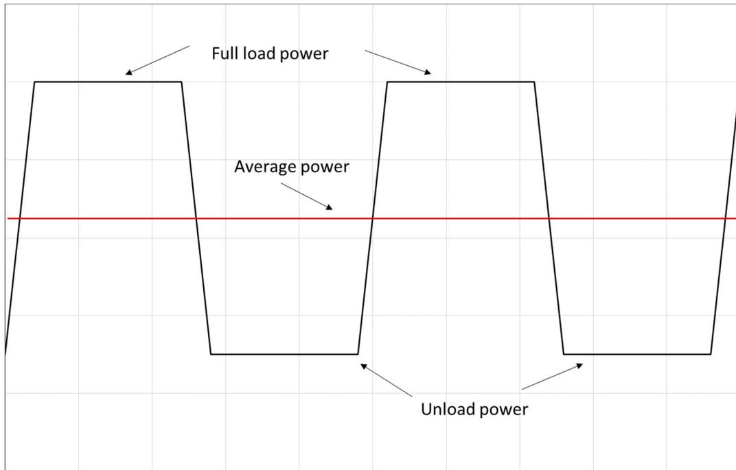
Figure 9.4 Compressor power profile when operating at 50% load
