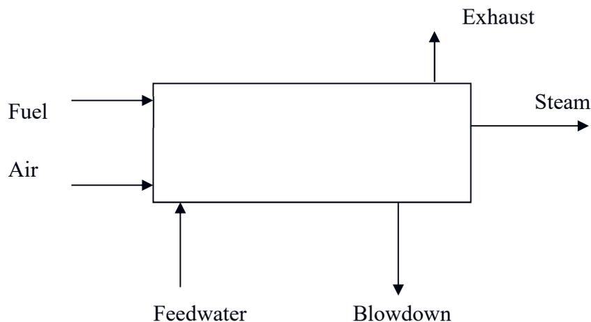
Figure 2.2 Main in-flows and out-flows for a typical boiler
