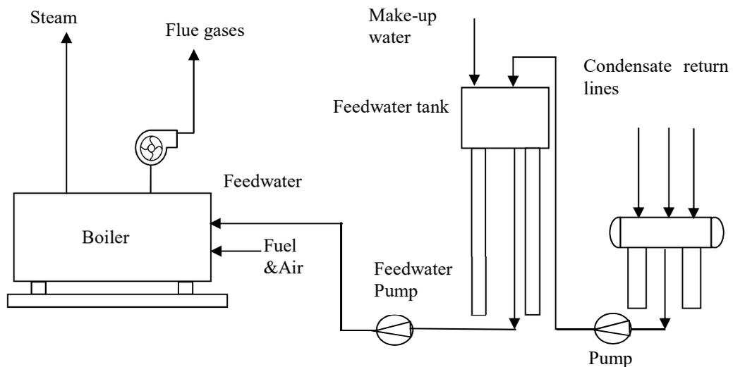
Figure 2.1 A typical boiler system
