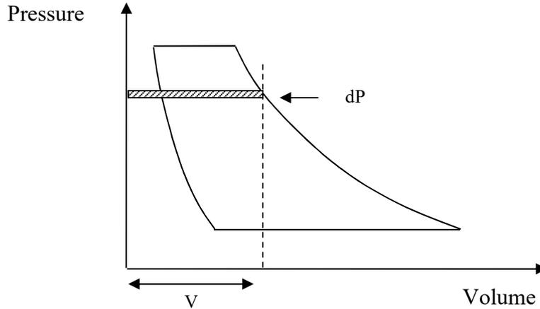
Figure 8.3 Work done in the compression process
