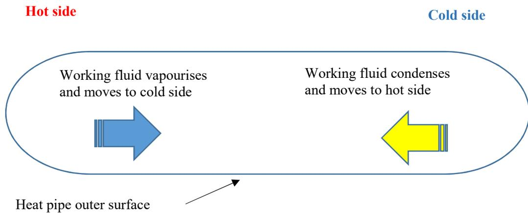
Figure 14.11 Working arrangement of a heat pipe
