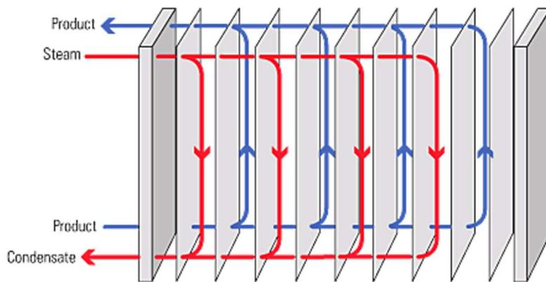
Figure 14.6 Arrangement of a plate heat exchanger (illustration taken from the Spirax Sarco website 'Steam Engineering Tutorials' at <http://www.spiraxsarco.com>)
