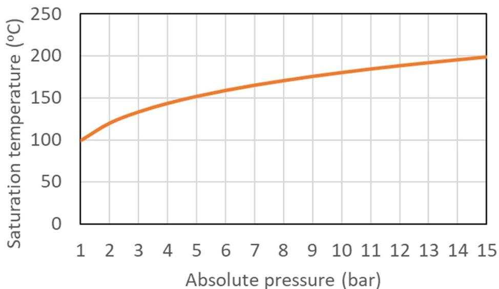
Figure 1.1 Steam saturation curve
