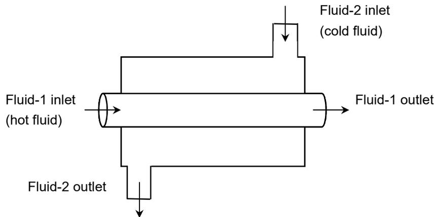
Figure 13.3 Arrangement of a counter flow heat exchanger
