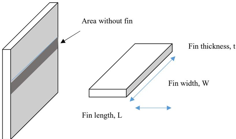
Figure 13.12 Illustration of area without fin
