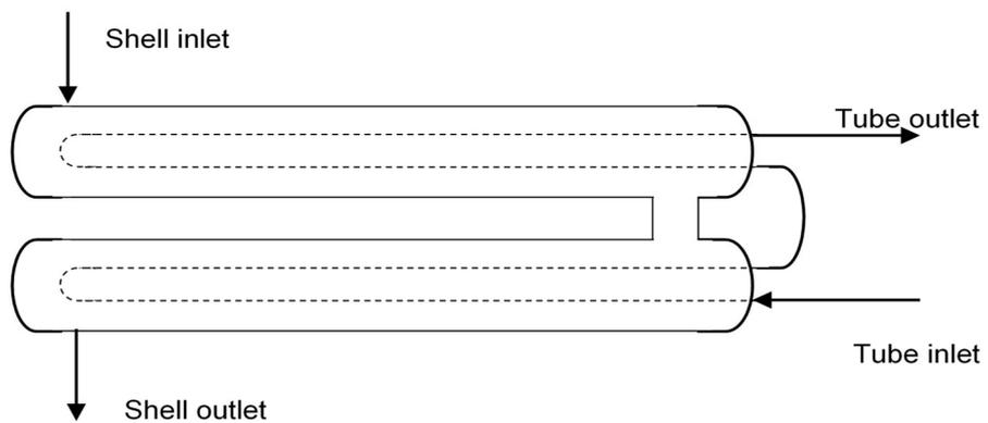
Figure 14.3 Two shell passes and four tube passes
