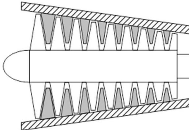
Figure 6.15 Cut-away of an axial-flow compressor
