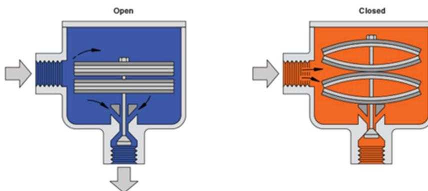
Figure 3.7 Operation of a thermostatic (bimetal) steam trap (images taken from the Spirax Sarco website 'Steam Engineering Tutorials' at <http://www.spiraxsarco.com>)
