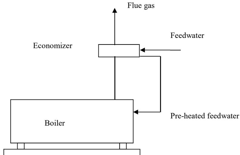
Figure 4.7 Arrangement of a typical economizer
