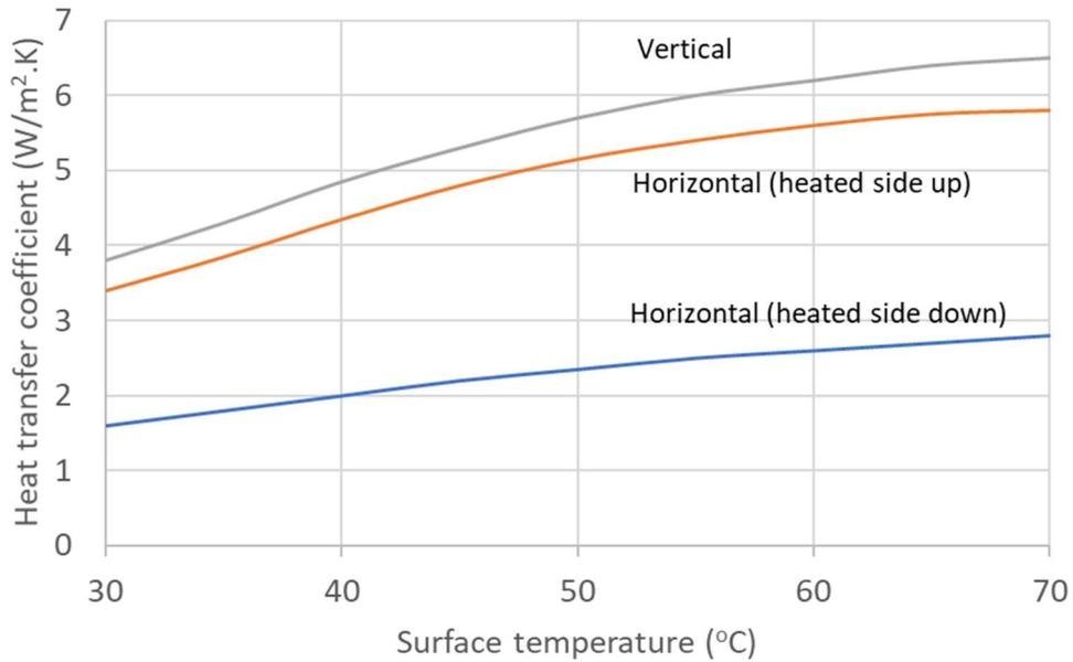
Figure 12.7 Heat transfer coefficient for natural convection
