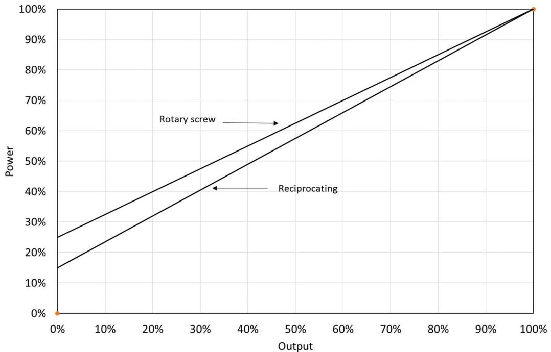
Figure 9.3 Output vs power for load / unload control
