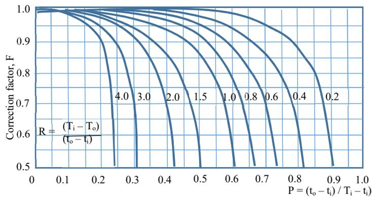
Figure 13.7 Correction factor F when one fluid is unmixed the other is mixed
