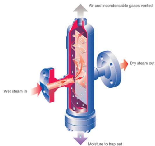
Figure 3.3 Cut-away of a steam separator (illustration taken from the Spirax Sarco website 'Steam Engineering Tutorials' at <http://www.spiraxsarco.com>)
