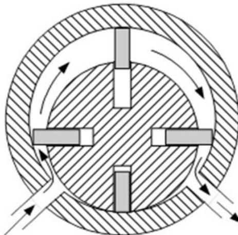
Figure 6.13 Cut-away of a rotary sliding-vane compressor
