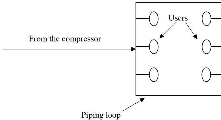
Figure 7.9 Distribution piping in a loop arrangement
