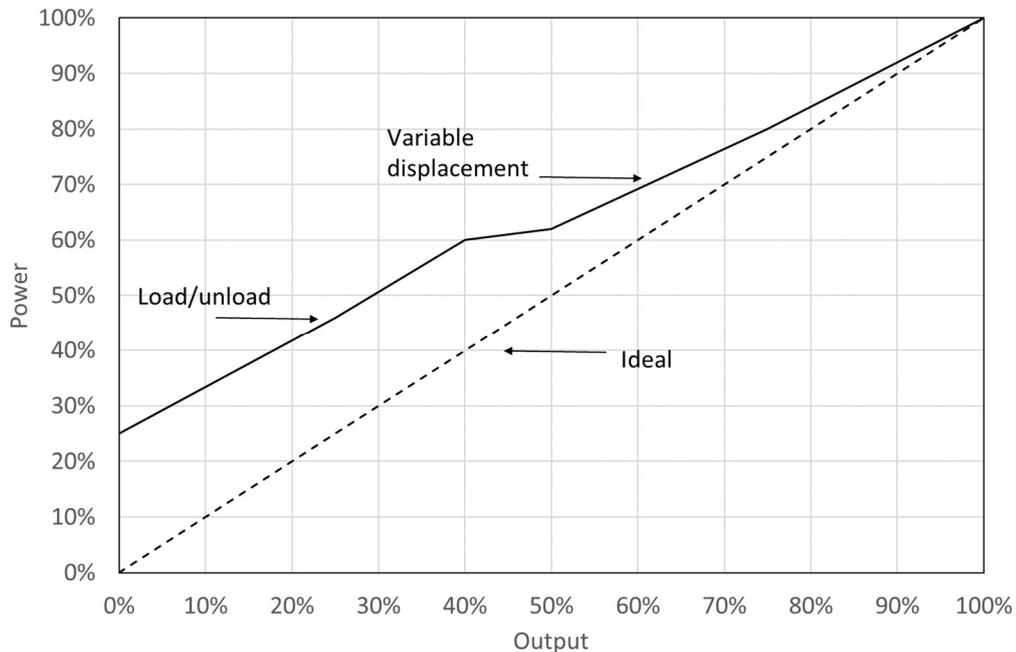
Figure 9.9 Output vs power for variable displacement followed by load / unload
