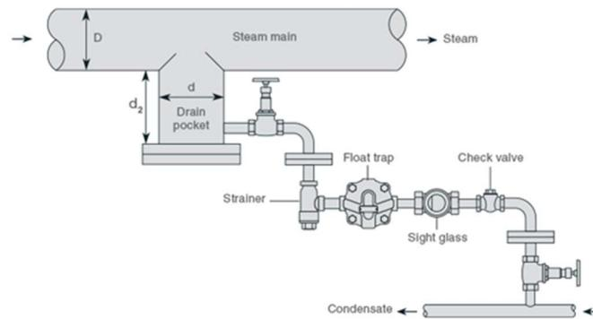
Figure 3.5 Arrangement of a steam drain pocket (illustration taken from the Spirax Sarco website 'Steam Engineering Tutorials' at <http://www.spiraxsarco.com>)
