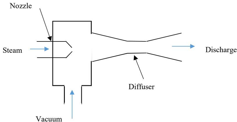
Figure 3.11 Arrangement of a steam ejector
