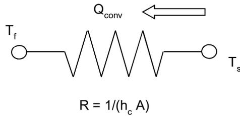
Figure 12.6 Ohm's law analogy applied to convective heat transfer
