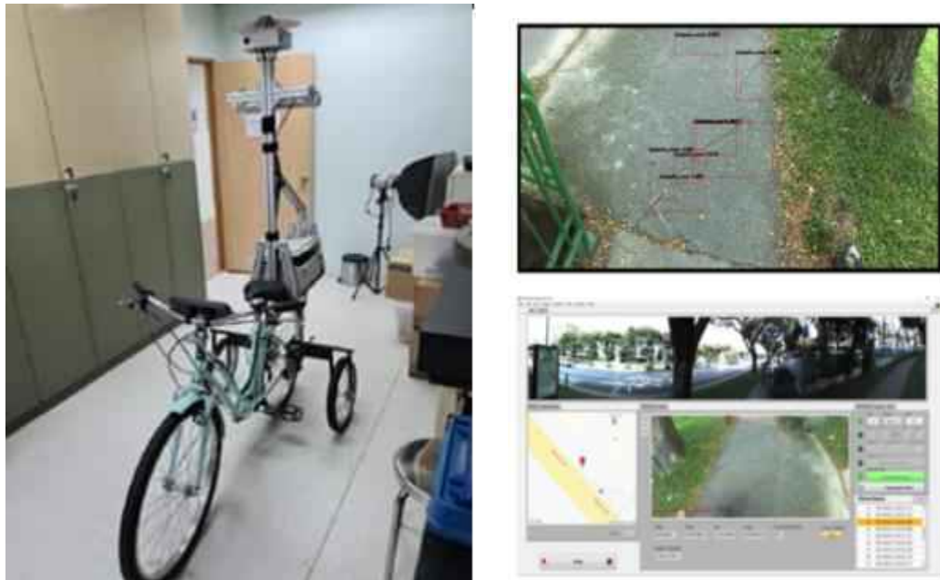
Figure 4.88: Camera mounted on bicycle for taking photos of the footpath
