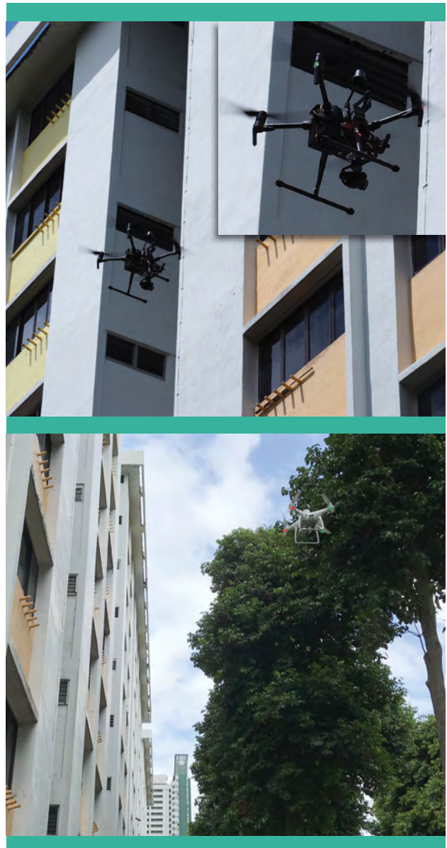
Figure 1: Drone performing building facade inspection.
