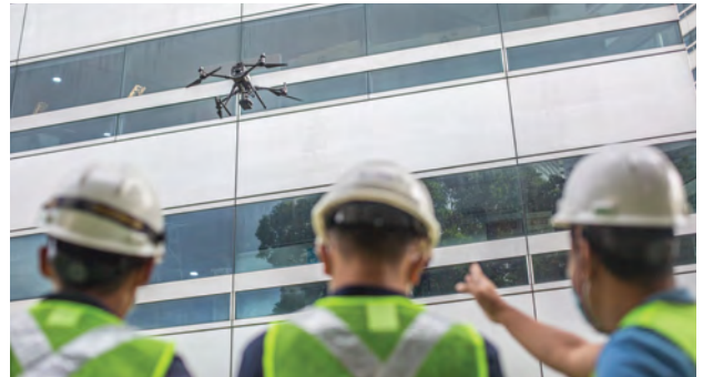
Demonstration of a drone inspecting a building façade. Image: BCA.
