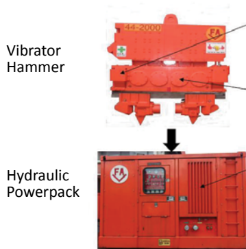
Components of a hydraulic vibratory hammer and how it works.
