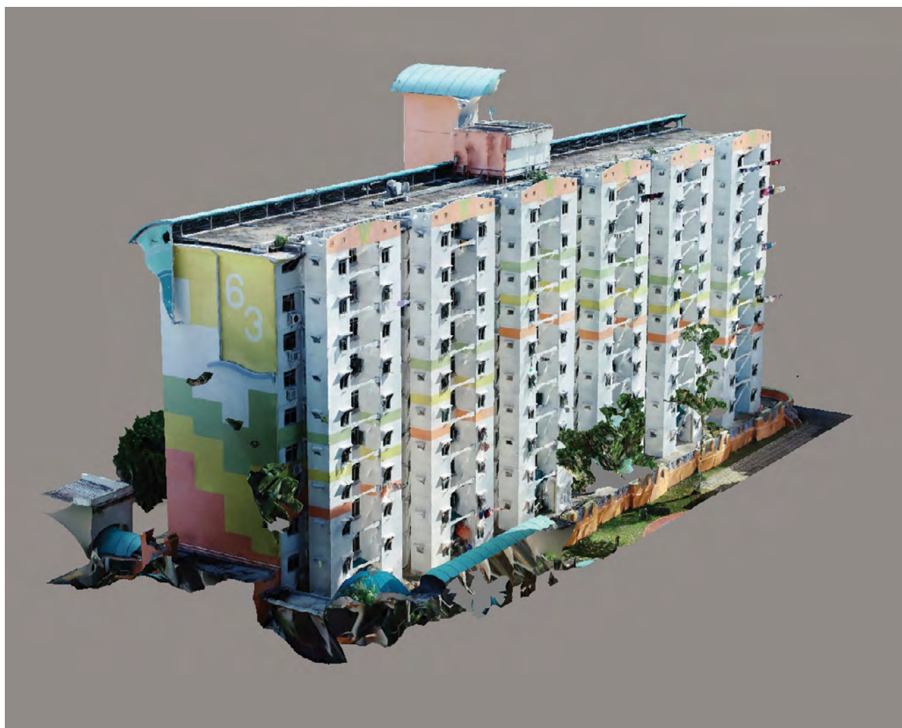
Figure 4: Reconstructed 3D model of a building inspected by a drone.
