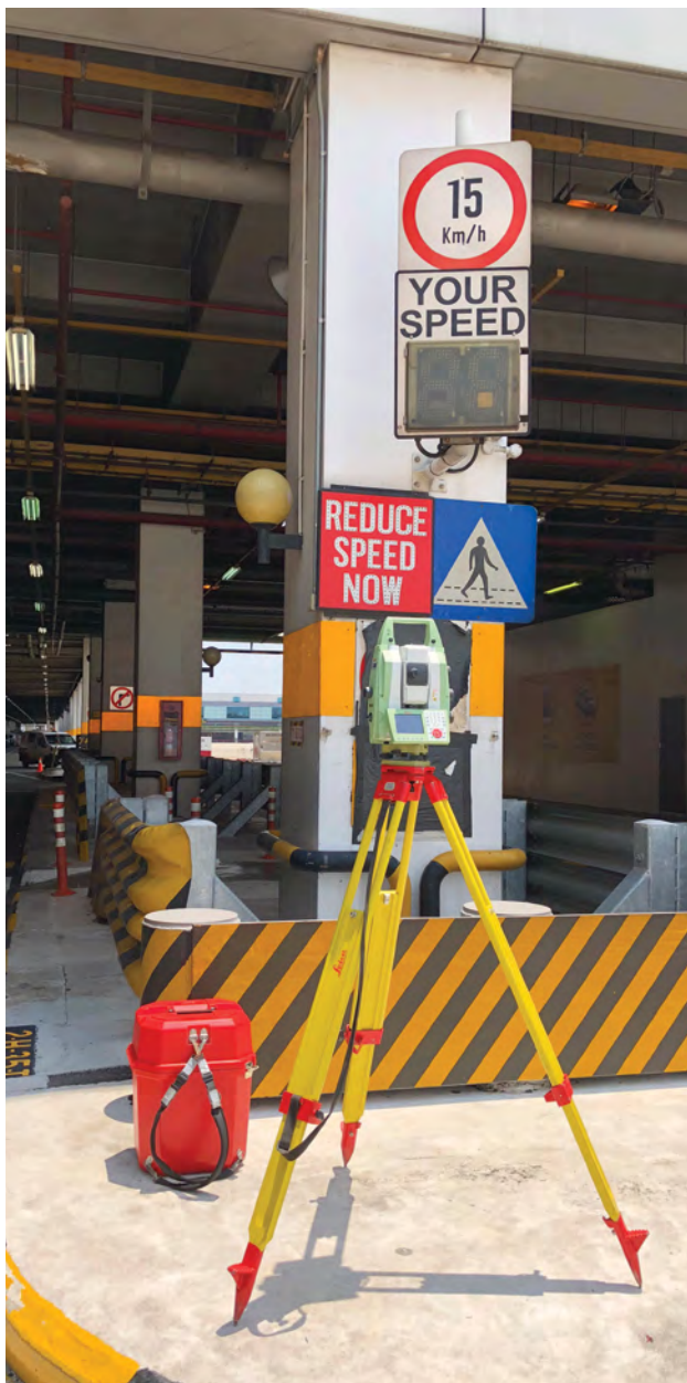
For the control surveying, JTRS used the Leica Nova TM50, six prisms and a Leica DNA03 digital level.
