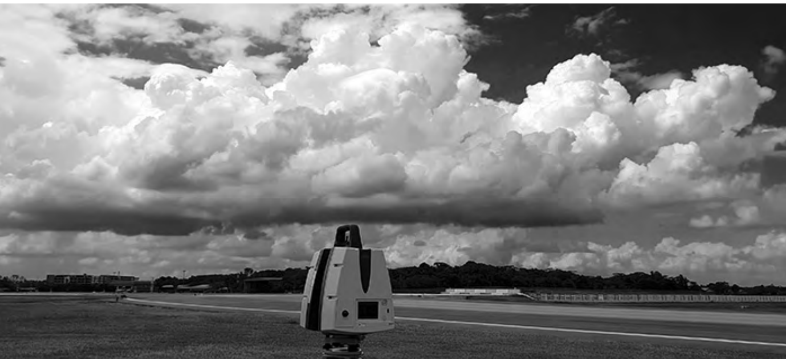
Leica ScanStation P40 was selected based on its ability to reach a high density, combined with good performance and reliability.
