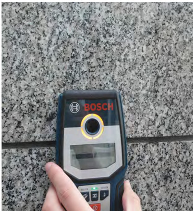
Using a metal detector to locate fixings.
