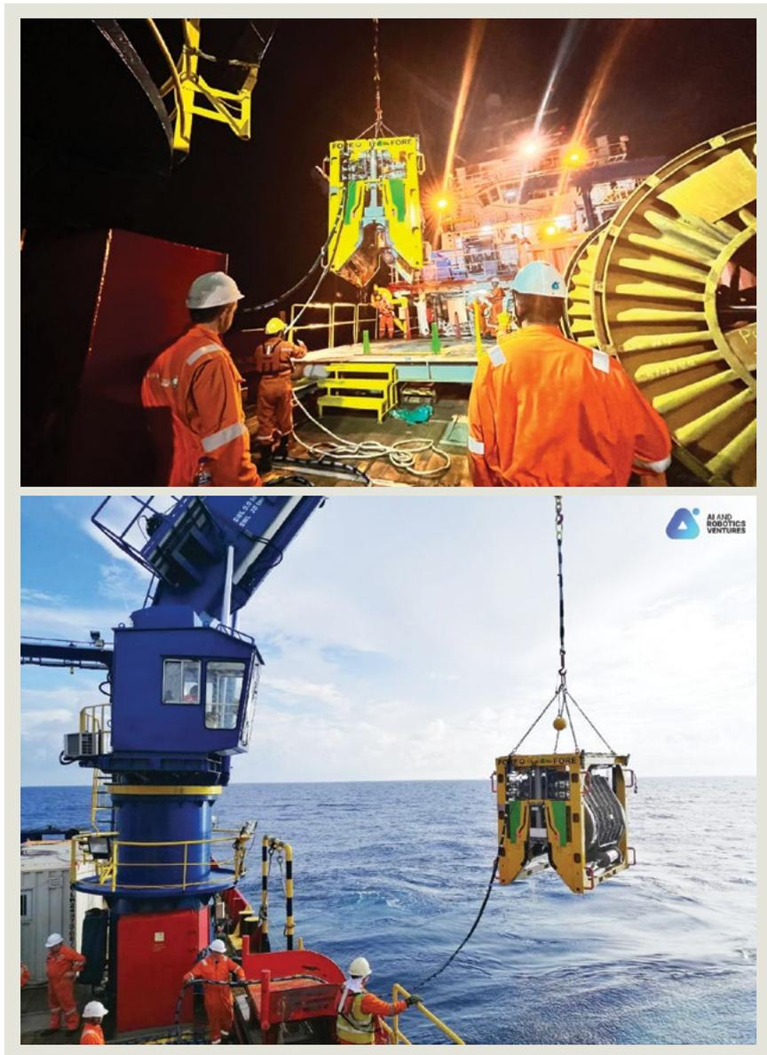
Nautilus is said to be the world's first subsea pipeline inspection and repair robot.
