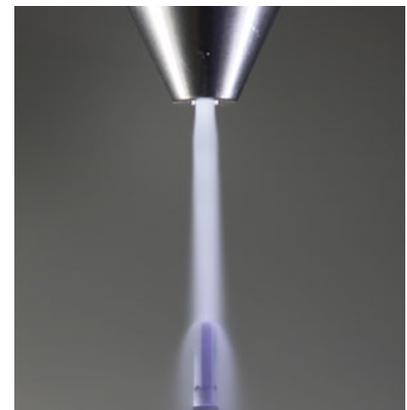
Thanks to the interaction of the effects of the quattroClean snow jet technology, particulate contamination down to the submicrometre range, as well as the finest filmic contamination, are removed reliably and consistently.
